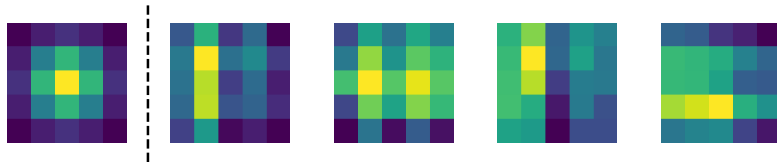
Figure 4.4: Example of low-pass filters extracted from the VGG41 baseline after insertion of BlurPool 5x5 (left) or TLPF 5x5 (right). In BlurPool all low-pass filters in the network are fixed by construction. In TLPF multiple different filters are learned.
