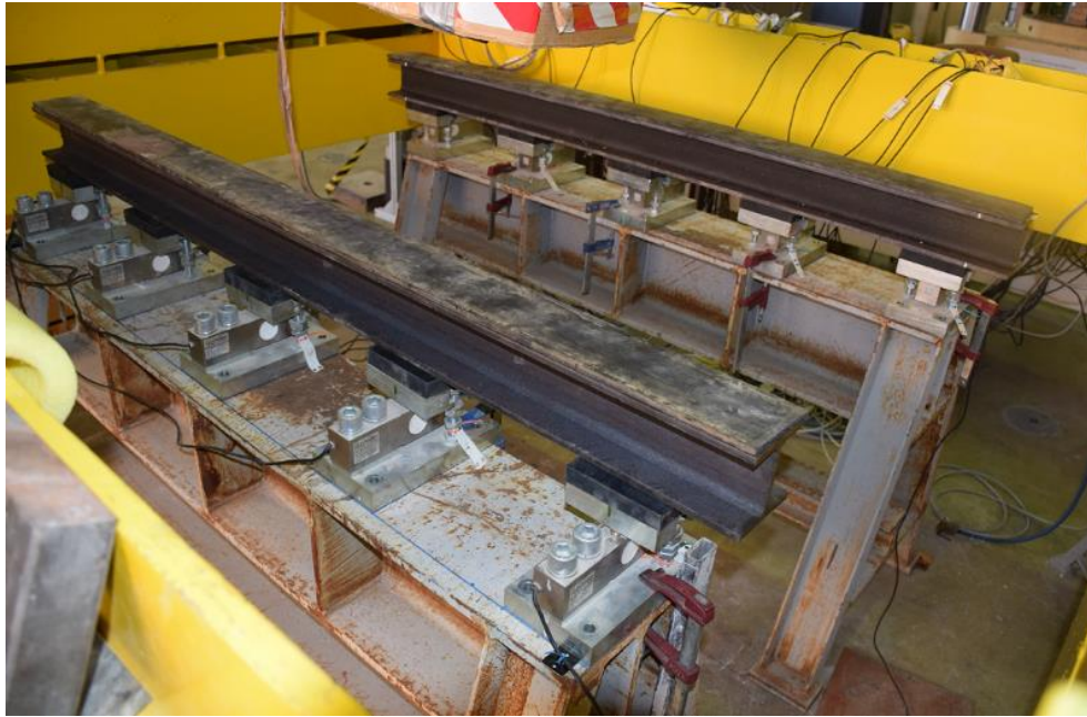
Figure 5.6: Support system of the tested specimens.
