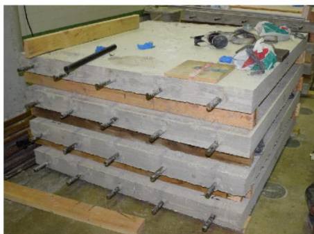
Figure 5.2: Position of post tensioning bars inside the slabs.
