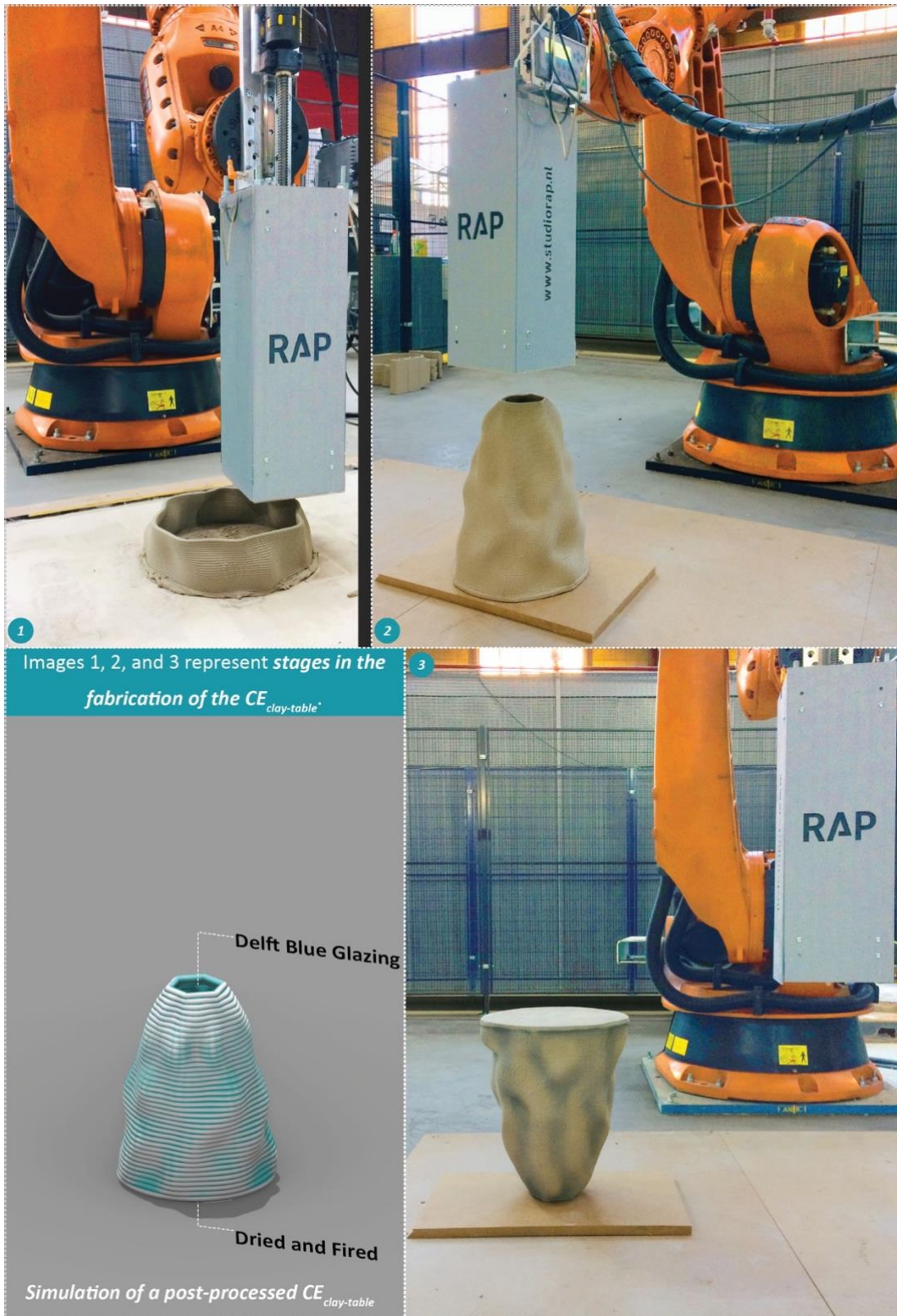
Figure 7.3 – Fabrication stages for the CE clay-table . Illustration, and photographs by Author (August 2020).
