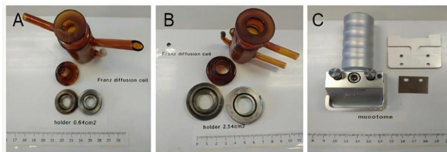
Figure 2. Tools used in permeation tests. (A): 0.64\ \text{cm}^2 Franz diffusion cell; (B): 2.54\ \text{cm}^2 Franz diffusion cell and (C): mucotome.
