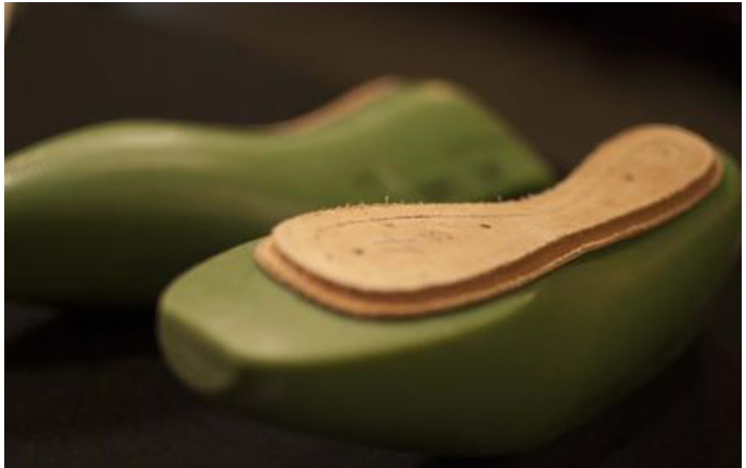
Figure 4.3 Clipping the sole on the last
