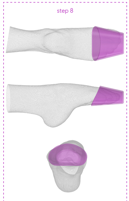
Figure 6.45 Step 8: Creating the surface of the platform and giving a thickness of 4mm.
