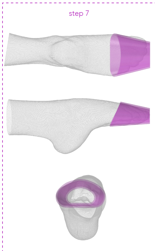
Figure 6.44 Step 7: Giving a thickness of 3mm to the box.
