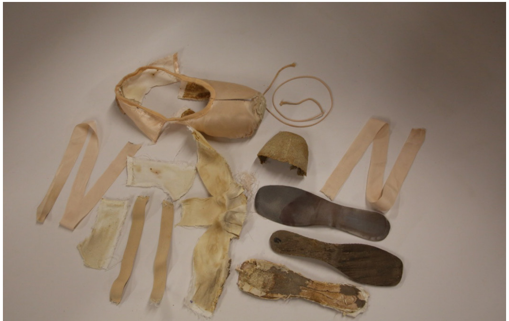
Figure 5.21 There are at least 13 different materials in the conventional pointe shoes.
