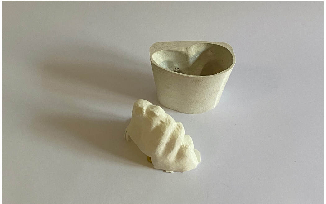
Figure 6.85 The first trial of the protective padding was made of a mold filled with liquid silicone.
