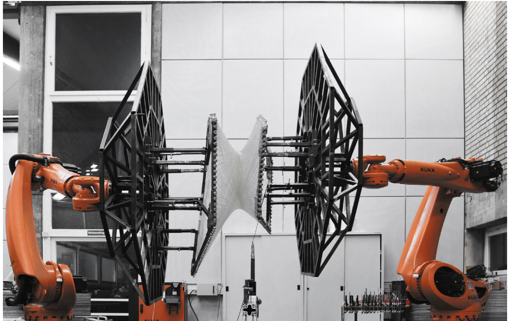
Figure 2.20. Synchronized robots winding a core-less filament for the creation of the Elytra Filament Robotic Pavillion by Achim Menges and ICD Stuttgart institute.
