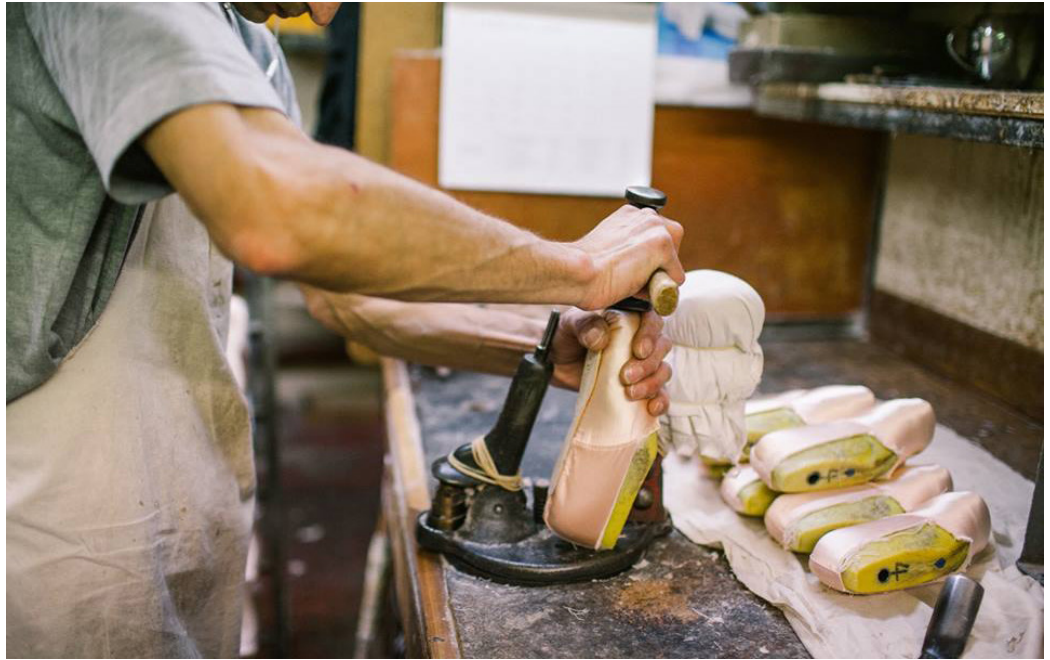
Figure 4.5 A shoemaker hitting the platform with a hammer to make the surface as planar as possible.
