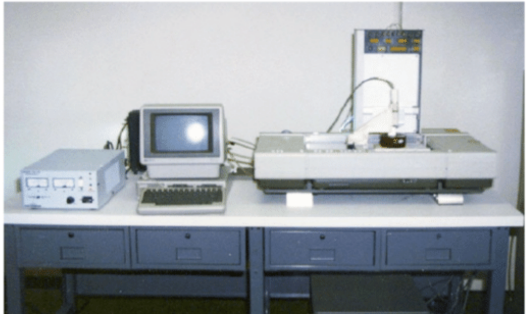
Figure 5.23 The Stereolithography Apparatus was invented by Charles Hull.
