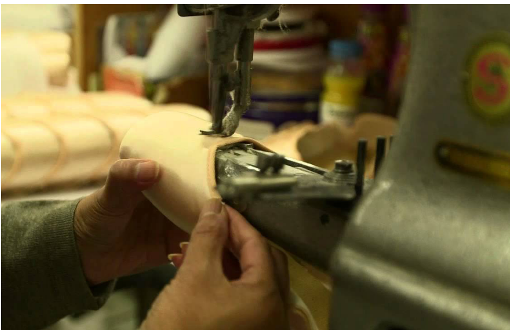
Figure 4.2 Sewing the satin for forming the outer shoe.
