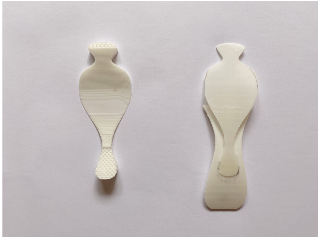
Figure 6.83 On the left can be seen the prototype printed with the layers in parallel with the axis of the folding and as it can be seen, it kept breaking even when trying to take off the support structure. On the right can be seen the prototype printed with the layers perpendicular to the axis of the folding which made it much more resistant..
