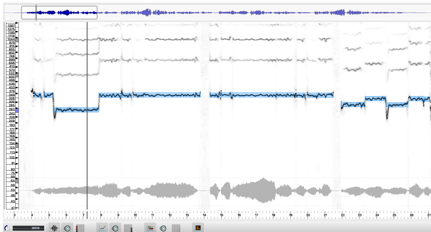
Figure 3.6: Screenshot of the Tony interface during the annotation process of the recording of an alto. The automatically extracted F0 contour is displayed in black, while the notes are depicted as blue horizontal lines.
