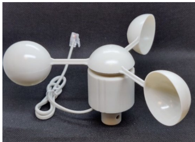
Fig. 7.27 - ADS Anemometer (image by author)
