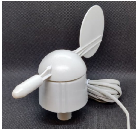
Fig. 7.29 - ADS Wind Vane (image by author)
