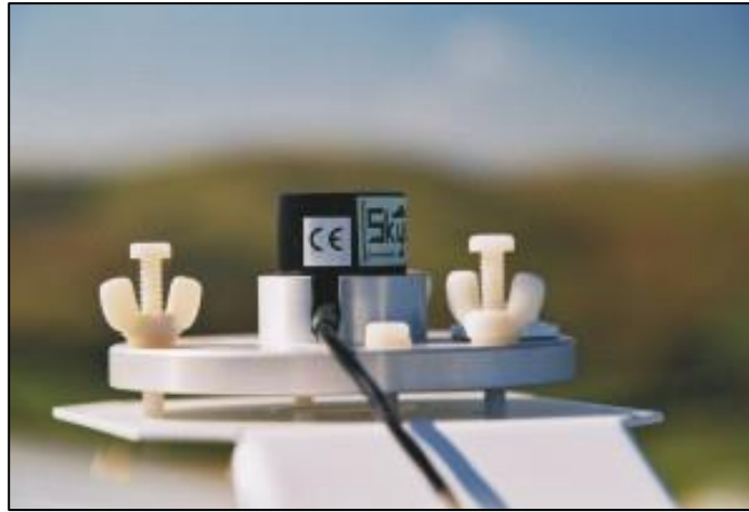
Figure 8. Pyranometer from SKYE Instruments Ltd.
