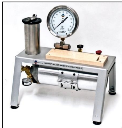
Figure 10. 3005-series portable plant water status console from Soil Moisture Equipment Corp.
