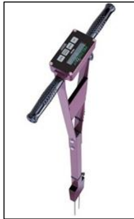
Figure 12. Fieldscout TDR 300 from Spectrum Technologies Inc.
