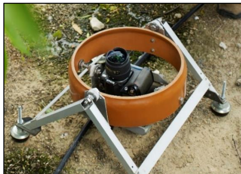
Figure 11. Digital camera on a self-levelling support.
