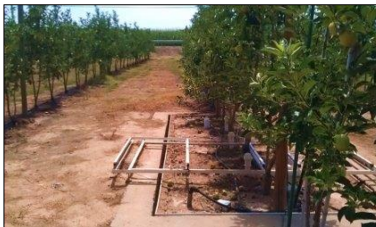
Figure 9. Weighing lysimeter located in Mollerussa Experimental Station.
