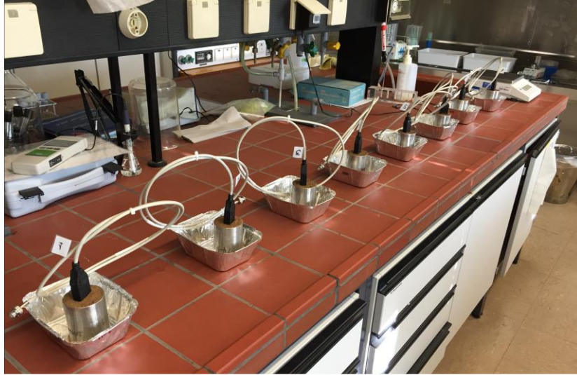
Figure 17. Local relationship between SWC and permittivity using TDR sensor.
