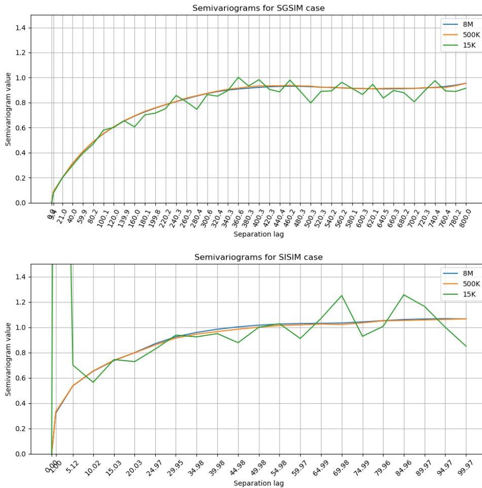
FIGURE 7.5: Sample semivariograms obtained using sgsim (top) and sisim (bottom) scattered data sets.
