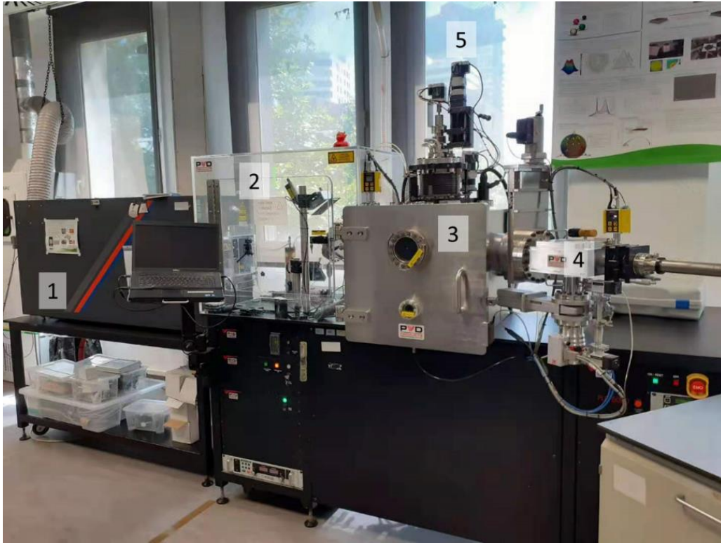
Figure 2.2 LA-PLD machine of PLD-5000 model from PVD Products® used for thin film deposition at IREC with the major components indicated: (1) laser excimer, (2) lens and mirrors, (3) vacuum chamber, (4) load lock chamber and (5) substrate motor, respectively.
