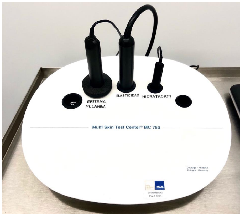
Figure 7. Probes of multi-probe device from left to right: pigmentation (erythema and melanin), elasticity and hydration probes.
