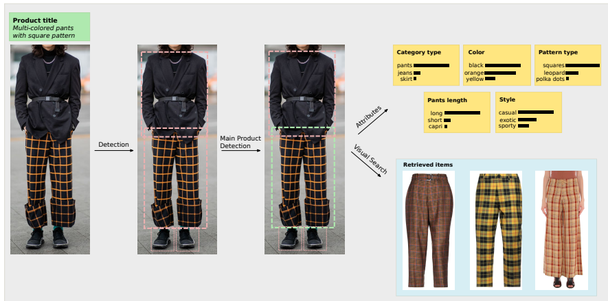
Figure 1.1 – Usual steps of a fashion product processing pipeline: fashion item detection, main product detection, attribute recognition and visual search.
