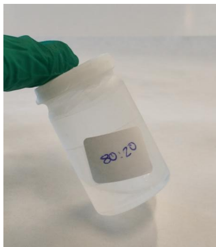
Figure S6. 80:20 ENB:DCPD mixture at -70^{\circ}\text{C} after 14 days. The blend presents fluidity and no phase separation.
