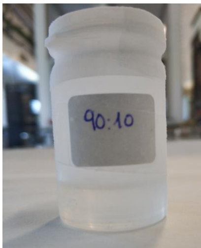
Figure S8 90:10 ENB:DCPD mixture at -70^{\circ}\text{C} after 14 days. The blend presents fluidity and no phase separation.
