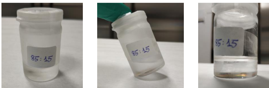
Figure S2. 85:15 ENB:DCPD mixture at -20°C after 14 days. The blend presents fluidity and no phase separation.
