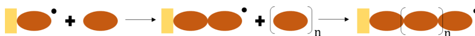
Scheme 1.2. Propagation process in the Chain-Reaction polymerization. The initiated chain with the free radical reacts with more monomers, bonding them and transferring the electron to the chain end.
