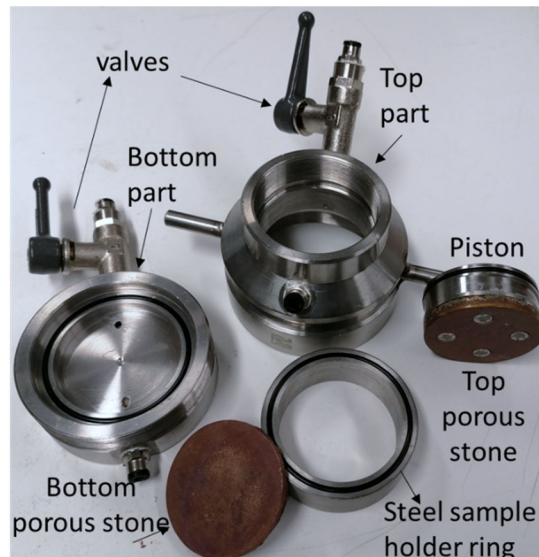
Figure 3-20. Parts of the isochoric cell. Isochoric cell. From Hoffmann (2005).
