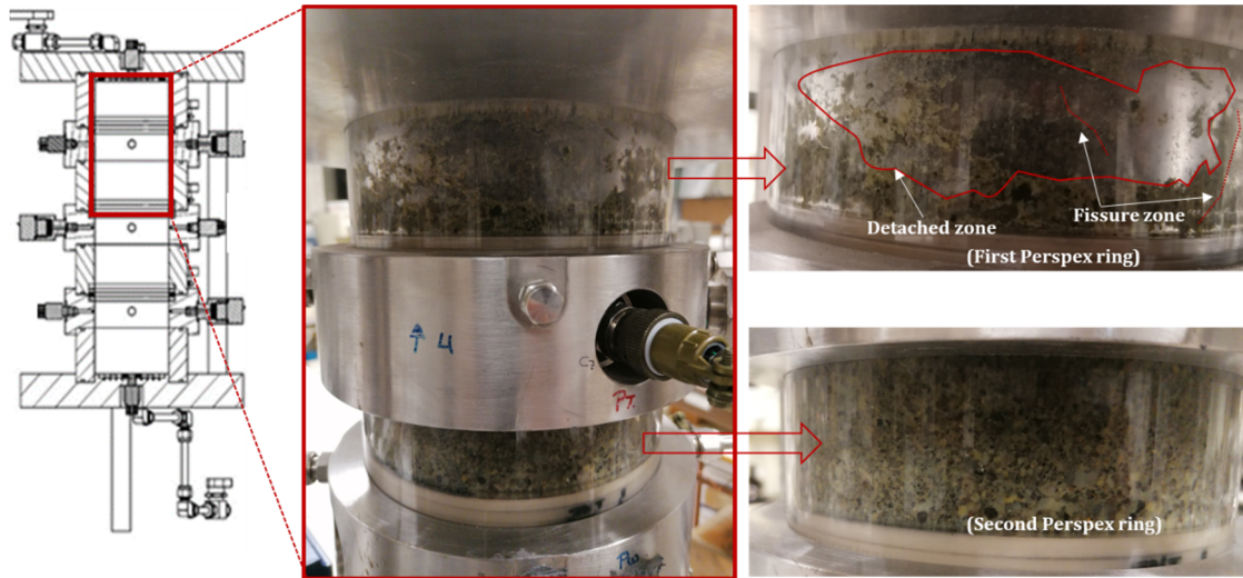
Figure 5-28. Second gas test with Perspex/bentonite interface problems in the top ring. Second ring with no discernable detachment or fissures.
