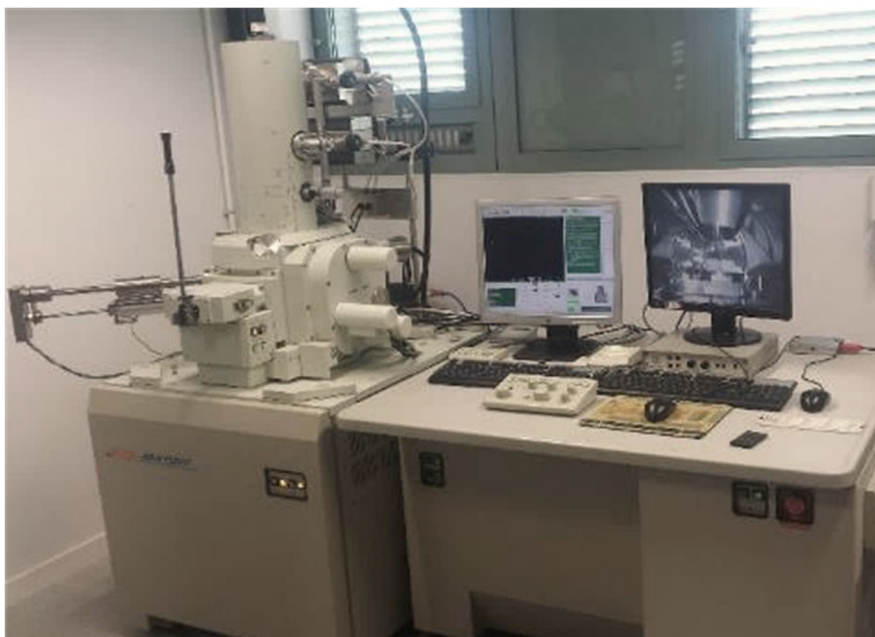
Figure 2-17. FESEM microscope (JEOL JSM-7001F).
