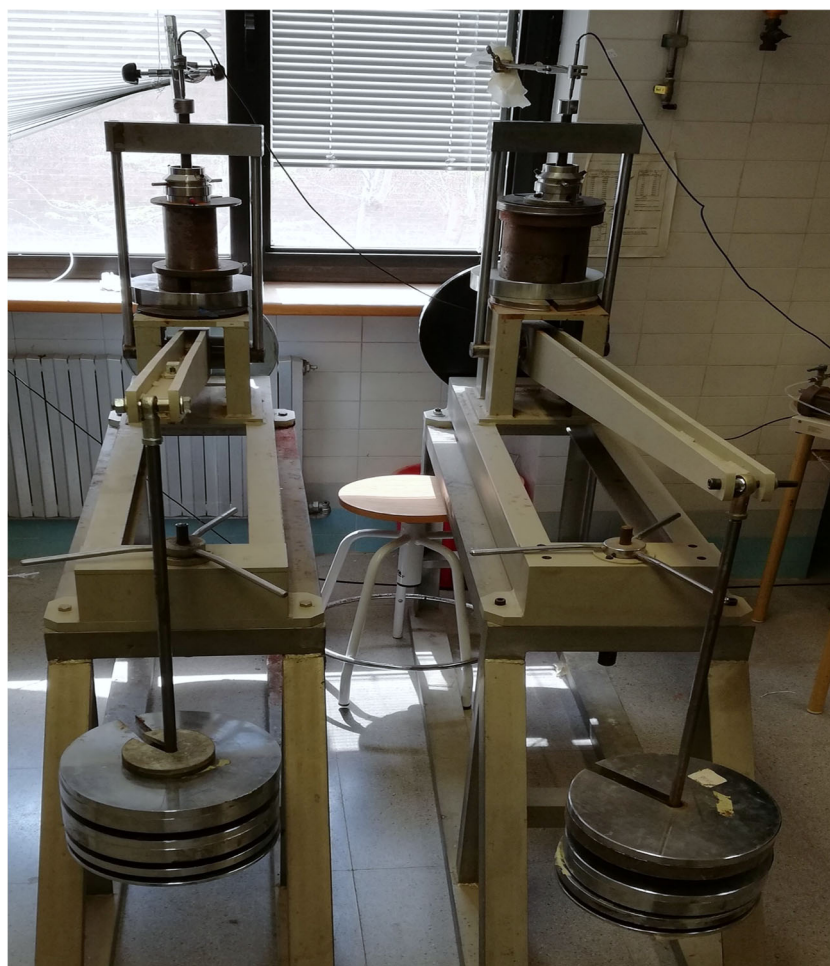
Figure 3-7. Setup for oedometer tests.
