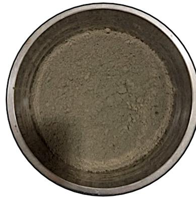
**Figure 3.2.** Raw Calcium Aluminate Cement.
