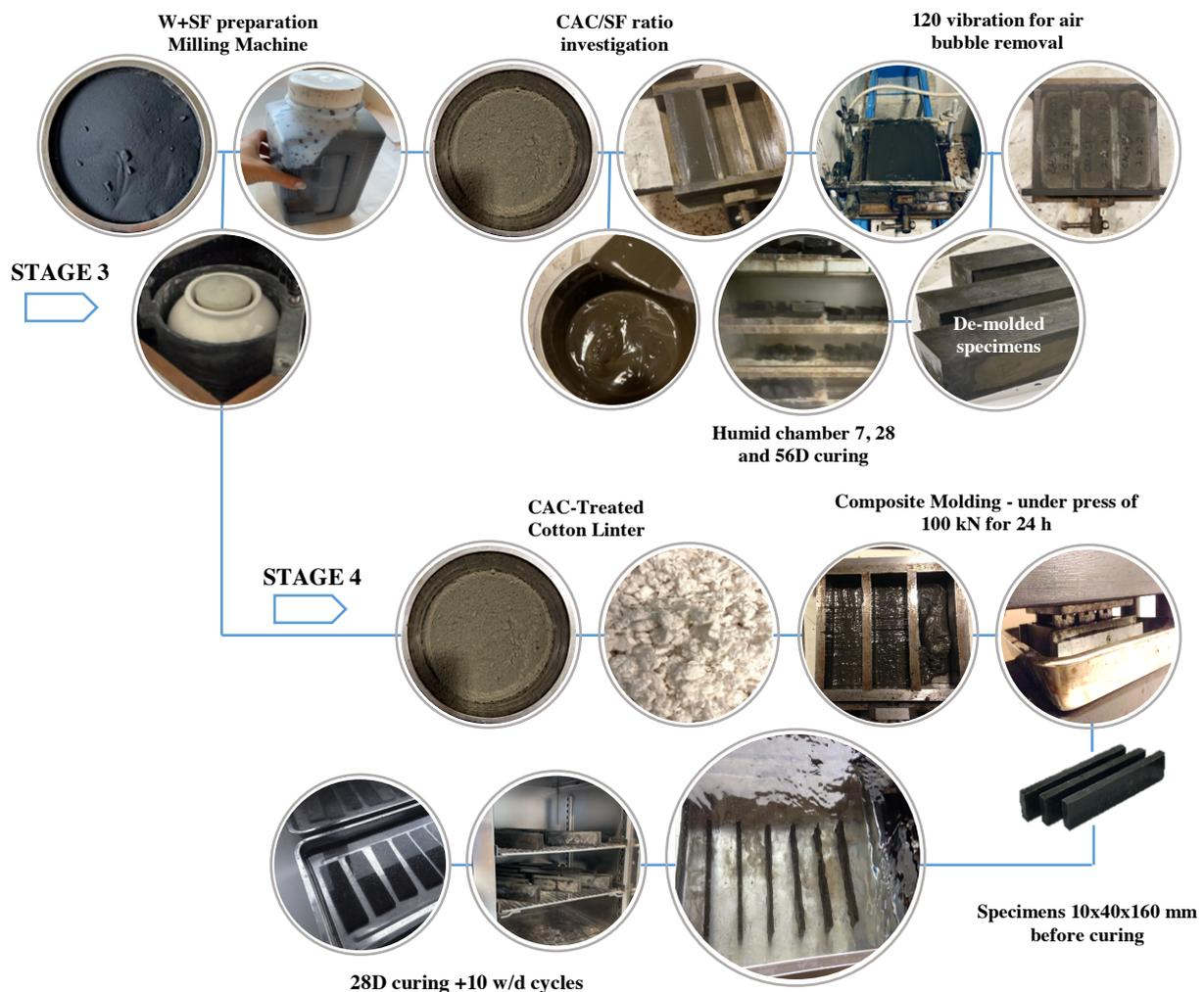
Figure 3.7. The schematic representation of the specimen production and equipment for the 3<sup>rd</sup>-4<sup>th</sup> experimental stages.
