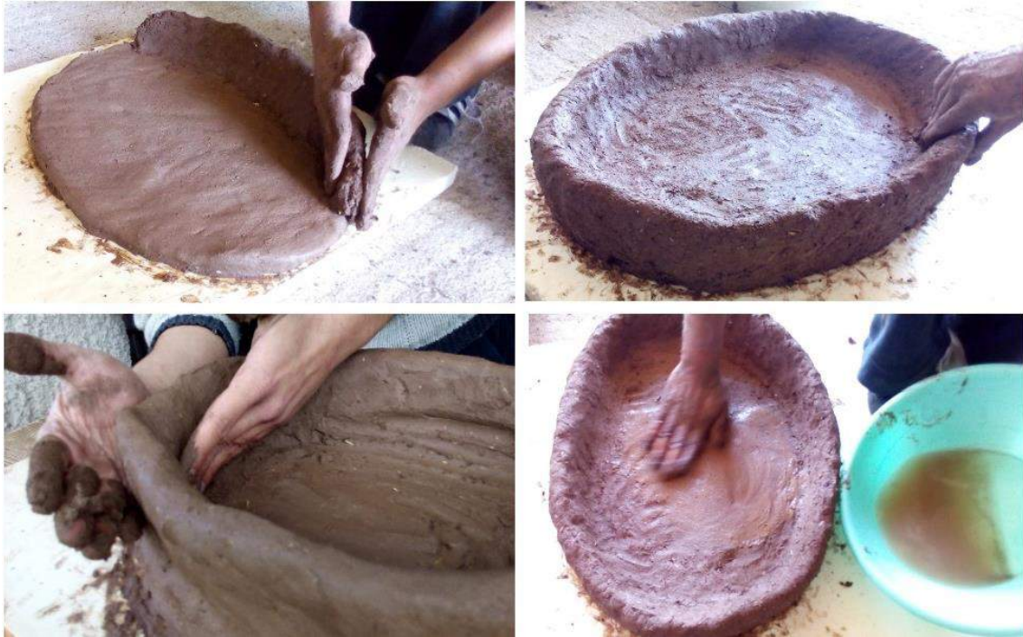
Fig. V.2 Shaping (on the right) and surface treatment (on the left) phases.
