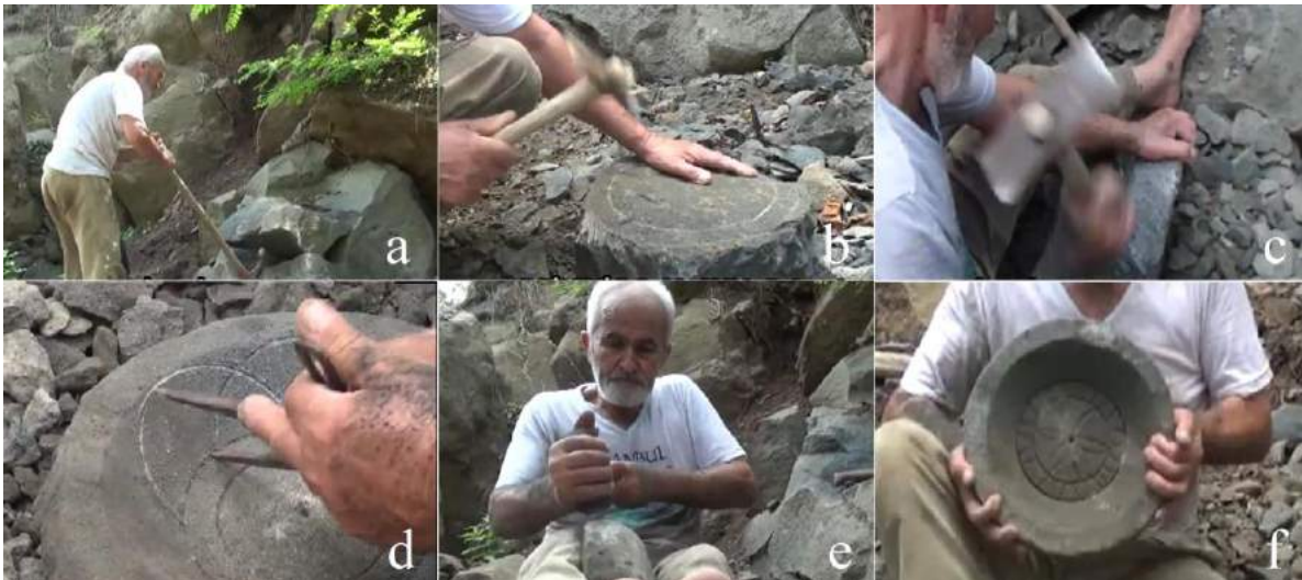
Fig. IV.12 Steps of the production sequence of a taş pileki in the Çarşamba district, Samsun. (elaborated from https://www.youtube.com/watch?v=pjPUf5mdljo )
