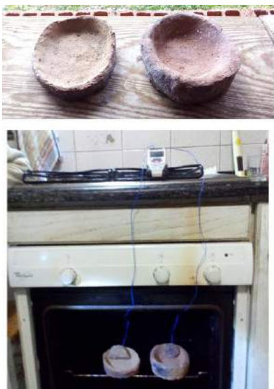
Fig. V.23 Reaction of a thinner and a thicker bowl to heat.
