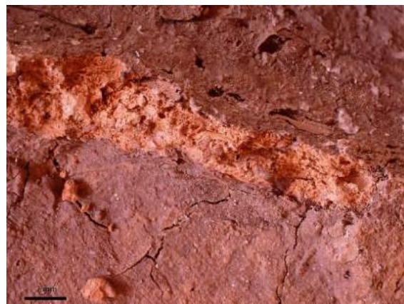
Fig. VI.24 Rip trace due to baking on the surface of levanzo.
