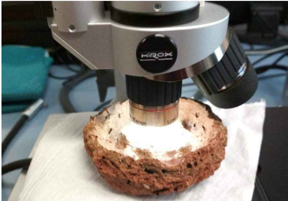
Fig. VI.13 Analyzing small replica under Hirox RH-2000 microscope
