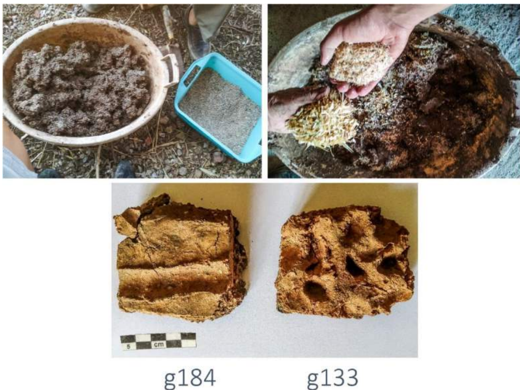
Fig V.22 Weight comparison between a mineral and plant tempered HT.
