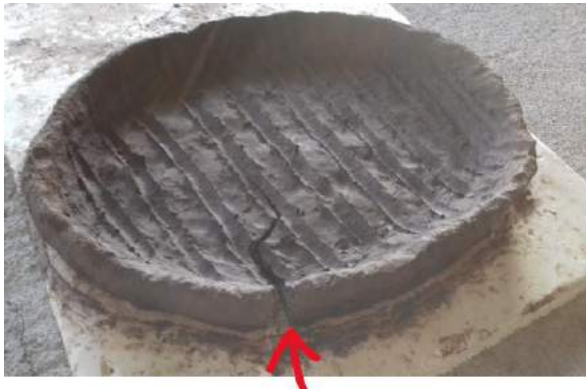
Fig. V.21 Cracked mineral tempered replica of HT
