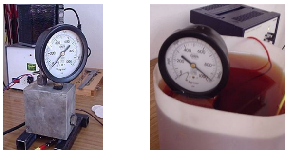
Figure 4.1: Closed single cell tested up to 950 bar.
