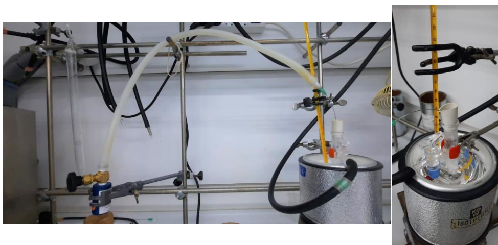
Figure 4.23: Set-up for the trifluoromethylation reaction. Left: general setup used to condense CF 3 I gas in the Schlenk tube. Right: zoom of the reactor cooled to condense the CF 3 I.
