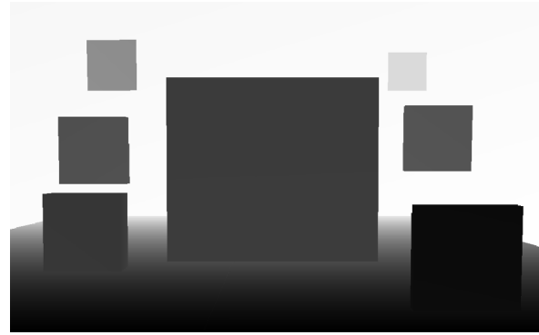
(b) Depth image generated by the simulation. As can be seen, the Ouchi marker is recognized by the simulator as a uniform plane. The Arco markers are placed in several depth levels.
