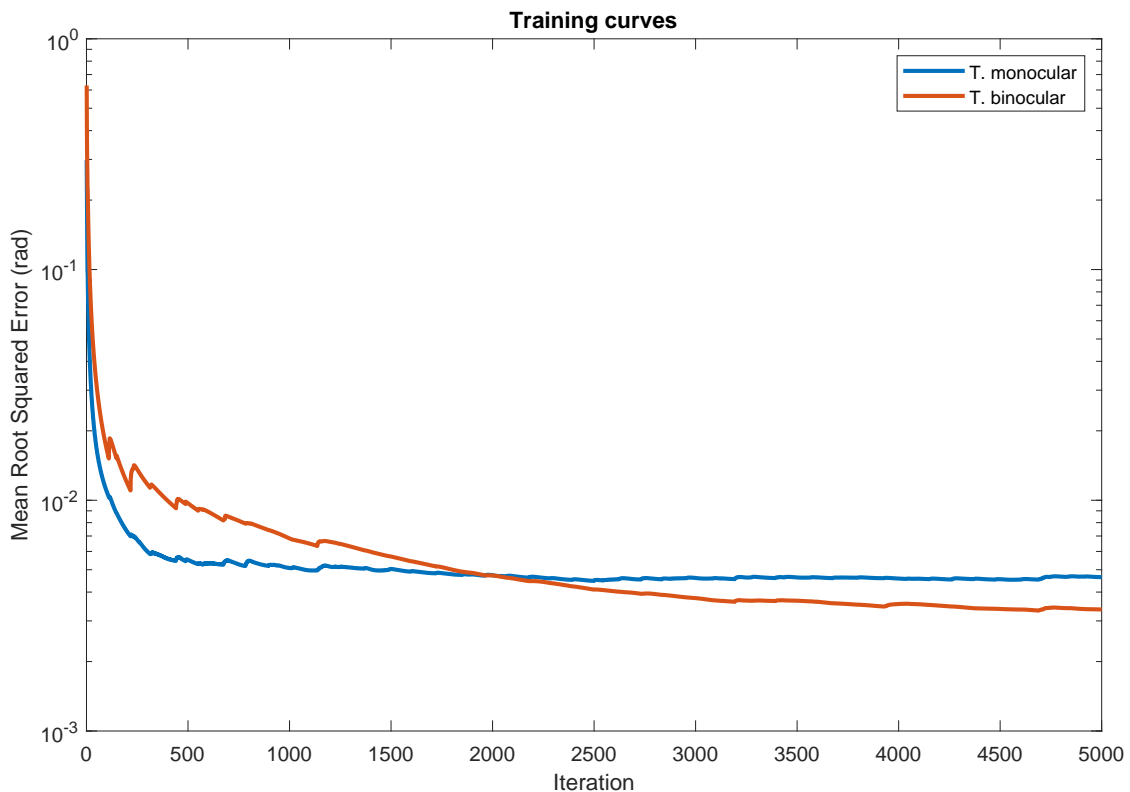
Figure 4.8: Learning neural networks curves for the proposed neural networks comparing the binocular and monocular training behaviour.
