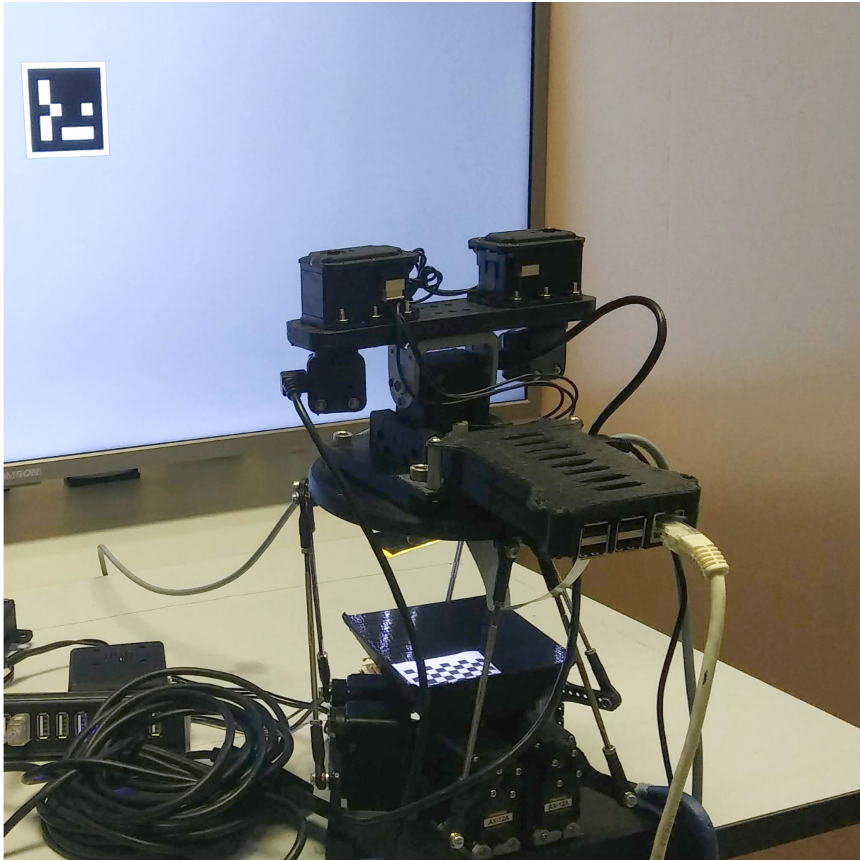
Figure 6.31: Final oculomotor-neck robotic system developed
