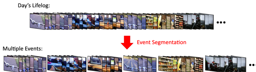
Figure 1.4: Example of temporal segmentation of an egocentric sequence based on what the camera wearer sees. In addition to the segmentation, our method provides a set of semantic attributes that characterize each segment.
