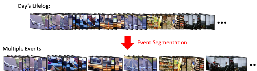
Figure 2.1: Example of temporal segmentation of an egocentric sequence based on what the camera wearer sees. In addition to the segmentation, our method provides a set of semantic attributes that characterize each segment.
