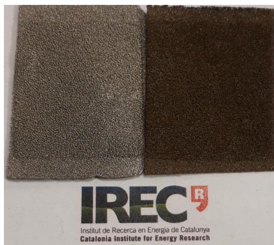
Figure 2.9. Photograph of an uncoated (left) and a coated Ni foam ( 10 \text{ cm}^2 ) with \text{CoFe}_2\text{O}_4 nanoparticles (right) after being 3 times immersed in the colloidal particle-containing solution.
