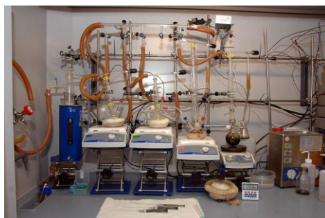
Figure 1.6. Colloidal synthesis Schlenk line set-up in FN group of IREC.
