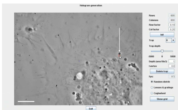
Figure 5. Manipulation of a 770\text{ nm} subcellular structure (endosome, lysosome, ...) near the nucleus of an NG-108 cell (Media 1). The arrow indicates the position of the vesicle that is moved by means of the holographic trap. Scale bar, 3\ \mu\text{m} .
