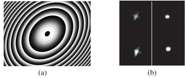
Figure 12. (a) Elliptical phase that corrects the aberration of Holoeye modulator. (b) Image of two optical traps without correction (left) and after correction (right).
