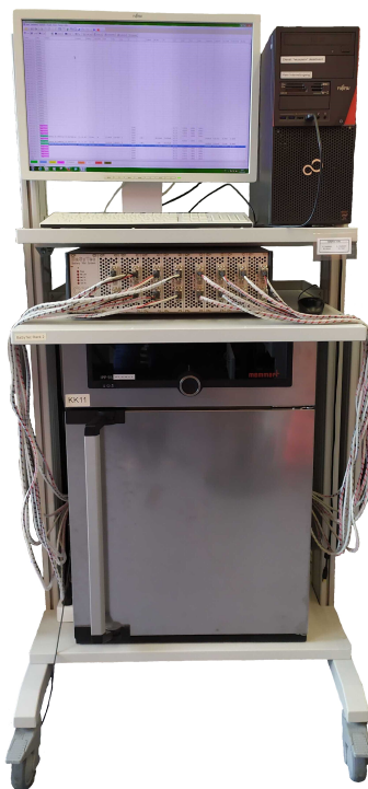
Figure A.5: Rack setup with BaSyTec cell test system and Memmert temperature chamber.
