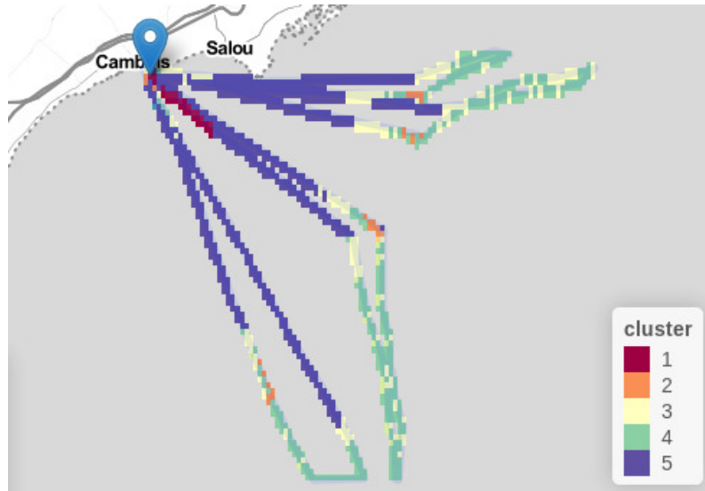
FIGURE 6.5. Example of status classification by clustering, on a trawling ship. Visualization tool at http://patrons.bsc.es .
