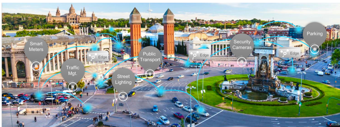
FIGURE 1.1. Example of different devices spread in a city that may be interconnected in the city of Barcelona. Intermediate edge devices may be set up to further process and aggregate the data produced in the devices. Image courtesy of David Carrera.
