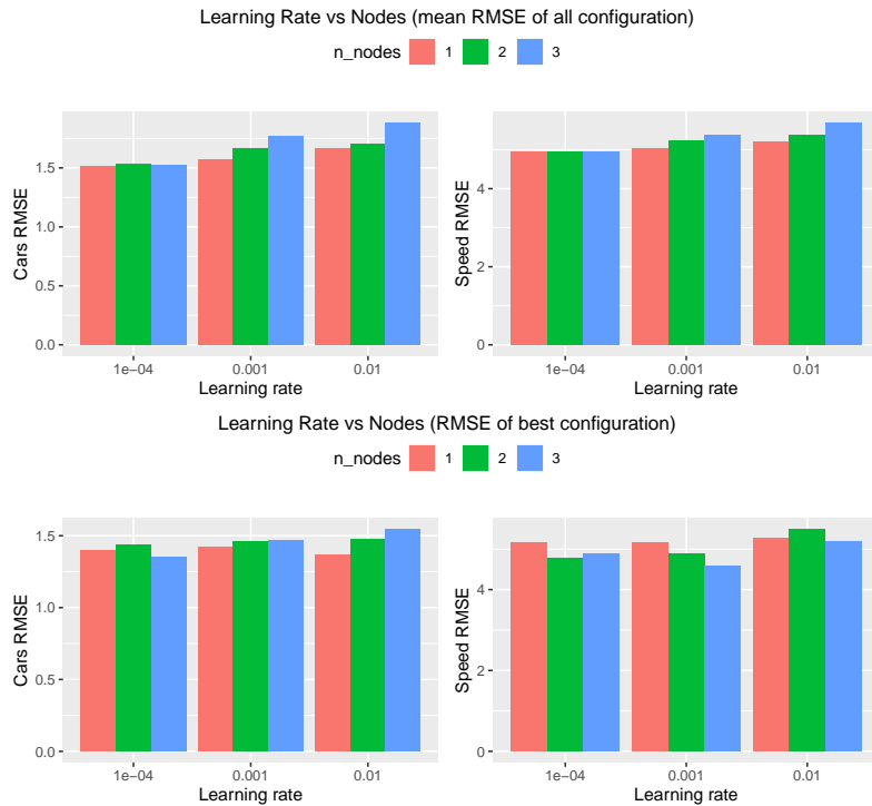
FIGURE 4.10. Comparison of the RMSE regarding the learning rate and the number of nodes (federated models) with (top) the average error of all the tested model configurations and (bottom) the best model configuration.
