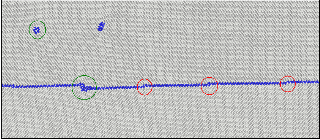
Figure 5.4: Snapshot of the interaction of the \mathbf{b}_{2/0} DPU with the \{112\} GB in W at T = 300 K. Defects are indicated with circles: red for EDiscs, green for \mathbf{b}_{-2/-4} GBD and \mathbf{b}_{2/0} reflected dislocation.
