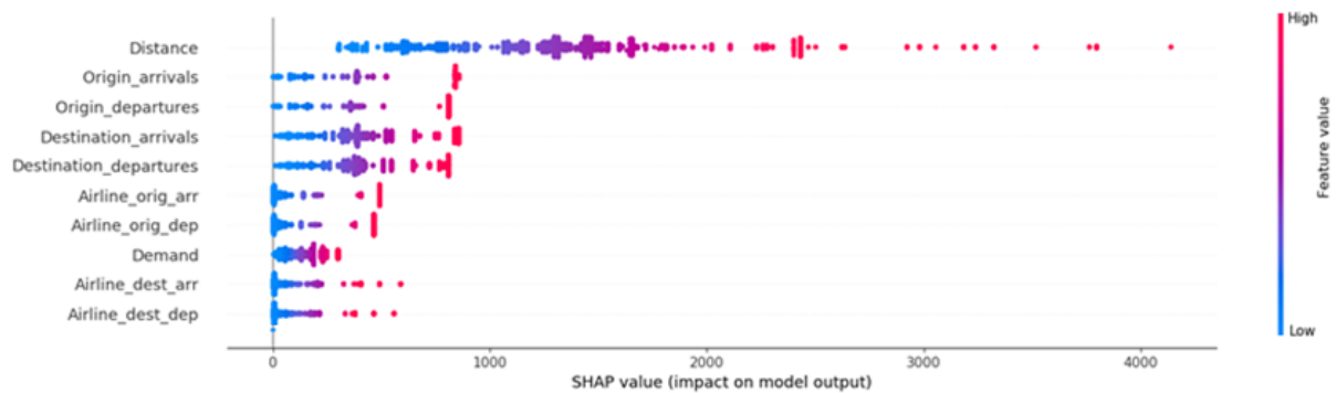
Figure IV-4: Shapley values for the 10 most relevant variables in the random forest TOW model. Variables are presented in order of the mean absolute Shapley value, each dot shows the impact of the feature on the prediction and the gradient color indicates the value for that feature in the corresponding prediction. Distance is, by far, the most relevant feature.
