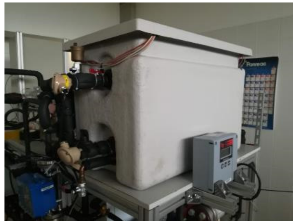
Figure 2. Latent heat TES.
