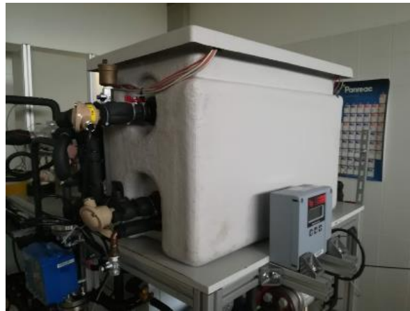
Figure 2-7. Latent heat TES.
