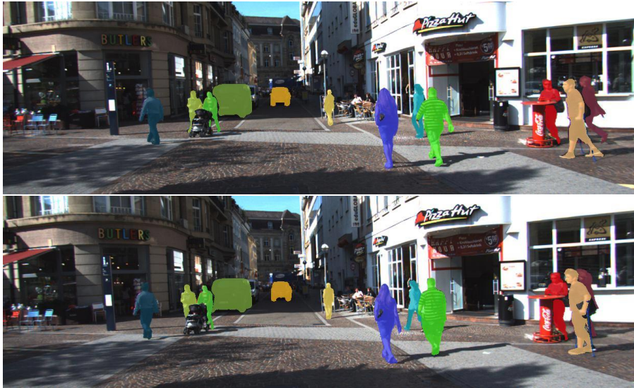
Figure 1.2: Multi-object tracking and instance segmentation output: detection, classification, tracking and instance segmentation of the object instances present along a street-level video sequence.
