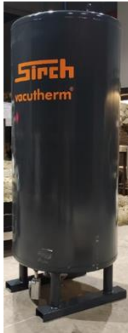
Figure 11: Picture of the stratified water tank at GREiA laboratory.
