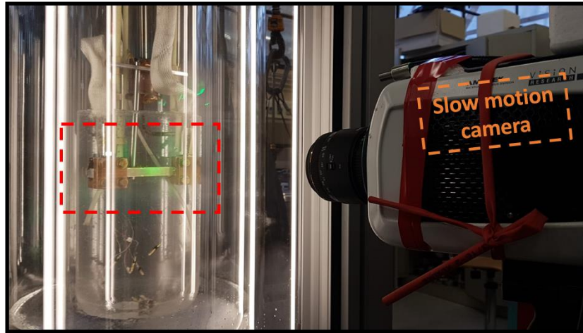
Figure 3.33: Picture of the slow-motion transport current set-up of Université Grenoble Alpes for filming the quench behavior of 2G HTS tapes in AC fault limitation tests. The transport current sample holder containing the sample is immersed vertically in a transparent cryostat to allow recording the footage.
