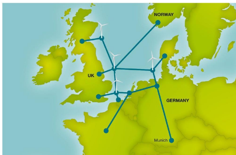
Figure 2.1: Estimated structure of the HVDC super grid in Europe by 2050.
