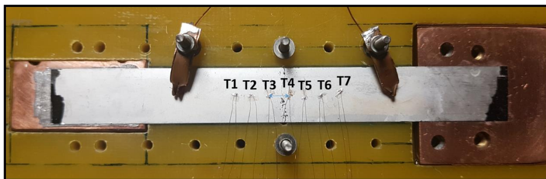
Figure 5.42: Yttria-CFD sample onto ICMAB's sample holder for transport current tests. Sample was mounted with 1 pair of voltage taps and 7 thermocouples for quench monitoring.
