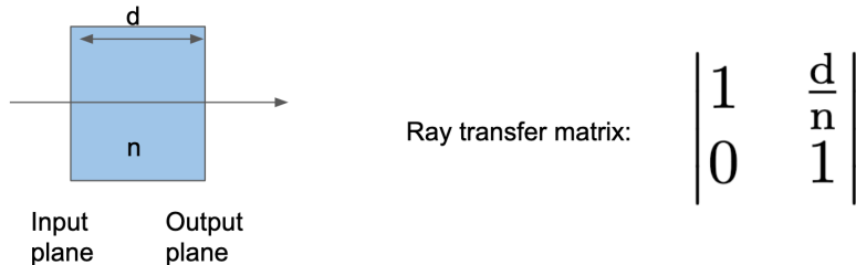
Figure E.5: Ray transfer matrix of rays passing through a dielectric material of index n and length d . The arrow represents the propagation direction.
