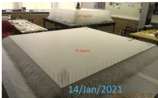
FIGURE 11.7: The final 56 layers for SuperFGD, divided in two groups of 11 and 45 layers.
