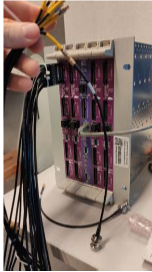
FIGURE 12.4: Picture of the final SAMPIC-based DAQ.
