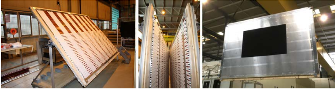
FIGURE 9.14: Pictures of: One half of a scintillating module being assembled (left), two half modules being brought together (middle) and a finished scintillating module covered by an Aluminum cover (right). Figure from Ref. [513].
