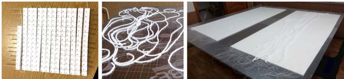
FIGURE 11.5: Steps for SuperFGD assembly. First (left) the fishing line is inserted sequentially in the array of cubes held together by the needles. Second (middle) 184 strings of 192 cubes are accumulated. Third (right) a full plane is made up joining together two half planes of 92 strings held together by spokes.
