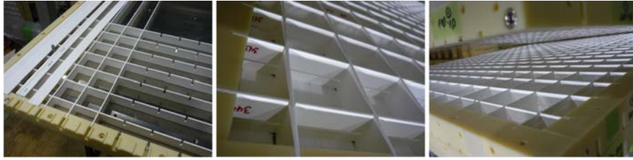
FIGURE 9.6: Pictures of the WAGASCI plastic scintillator 3D grid-like structure. The dimensions of each cell are 5 \times 5 \times 2.5 \text{ cm}^3 . Figure from Ref. [499].
