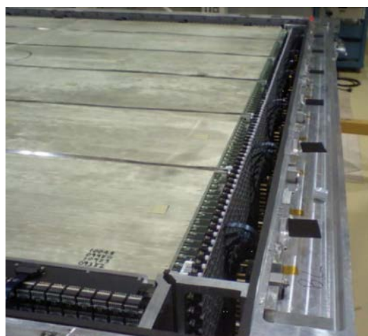
FIGURE 5.25: . Photograph of the XY modules inside the FGD1 dark box. Busboards carrying photosensors are mounted along all four sides of each module. Ribbon cables connect each busboard to the backplanes (not visible in this photo) on the sides of the dark box. Figure from Ref. [452].
