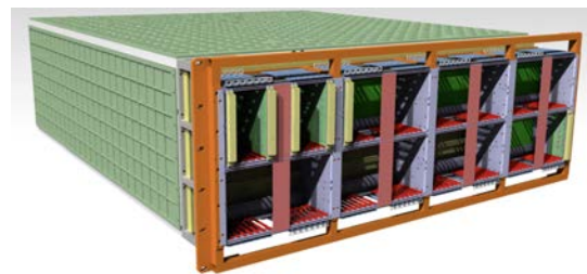
FIGURE 11.18: CAD drawing of the crates of one side installed in the SuperFGD box.
