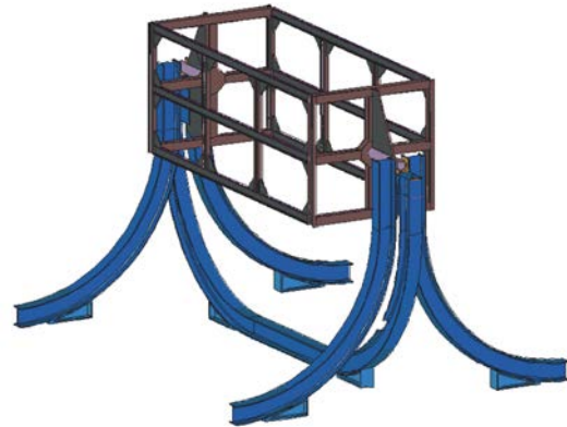
FIGURE 5.16: Sketch of the ND280 basket. Figure from Ref. [423].
