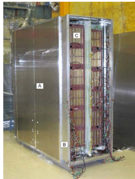
FIGURE 5.38: TPC outer box. A: one of the outer box walls; B: service spacer; C: one of the Micromegas modules inserted into the module frame. Figure from Ref. [456].
