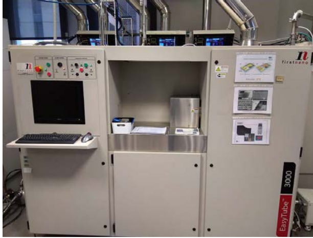
Figure 2.2: Illustration of the CVD system at IREC facilities ( FirstNano Easytube 3000 ) used for the fabrication of nanowires and nanofibers
