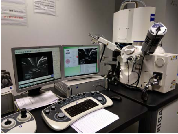
Figure 2.13: Scanning Electron Microscope (SEM) equipment (Zeiss® Auriga) with an Energy Dispersive X-ray spectrometer (EDX) (Oxford Instruments® INCA) used at the IREC facilities for the morphological and compositional analysis of the fabricated nanowires and microstructures. The equipment can produce acceleration voltages from 1.5 to 20 kV.
