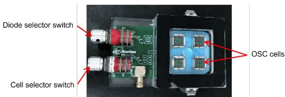
Figure 2.8 Sample-holder used to place the studied devices for the transportation and measurements outside the glovebox.
