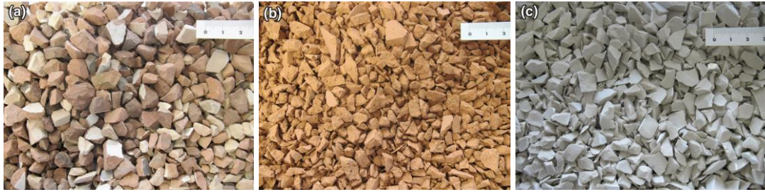
Fig. 2.1 The ceramic waste used as a recycled aggregate. Coarse fraction: a) tile ceramic waste, TCW; b) red clay brick, RCB; c) ceramic sanitaryware, CSW
