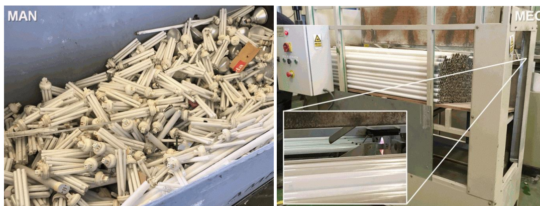
Fig. 4.2 The original spent fluorescent lamps: a) Manually processed; b) Mechanically processed.
