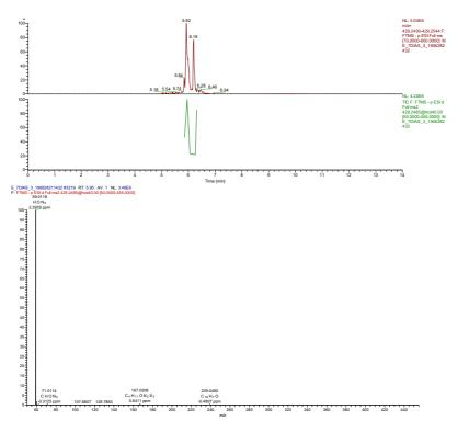
**Figure S15.** Extracted ion chromatograms (top: full MS, down: full MS<sup>2</sup>) and MS<sup>2</sup> spectrum of m/z 429.2486 (TP430).
