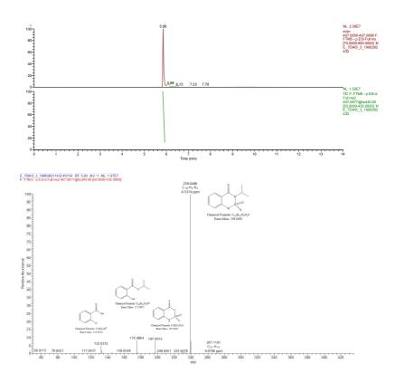
**Figure S12.** Extracted ion chromatograms (top: full MS, down: full MS<sup>2</sup>) and MS<sup>2</sup> spectrum of m/z 407.0676 (TP408).
