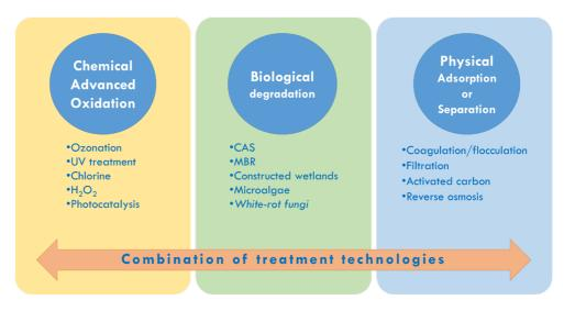
Figure 1.4. Scheme of the most typical processes involved in wastewater treatments.
