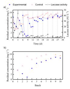
Fig. 6. Removal of bentazone by *T. versicolor* in sequencing batch TBR under non-sterile conditions. a. Time-course of bentazone variation during the treatment; b. The final concentration of bentazone in each batch.
