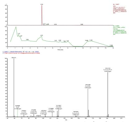
**Figure S19.** Extracted ion chromatograms (top: full MS, down: full MS<sup>2</sup>) and MS<sup>2</sup> spectrum of m/z 191.0119 (TP192).
