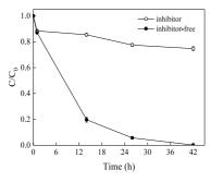
Fig. 3. Influence of the cytochrome P450 inhibitor 1-aminobenzotriazole on the degradation of bentazone by *T. versicolor*. C represents the residual concentration of bentazone in the sample (mg L<sup>-1</sup>), and C<sub>0</sub> corresponds to the concentration of bentazone at the beginning of the experiment (10 mg L<sup>-1</sup>). Values are the mean and standard deviation of three replicates.
