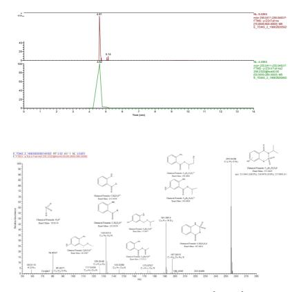
**Figure S3.** Extracted ion chromatograms (top: full MS, down: full MS<sup>2</sup>) and MS<sup>2</sup> spectrum of m/z 255.0445 (TP256, OH-BTZ).
