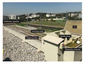
Figure S1. Pilot outdoor photobioreactor.
