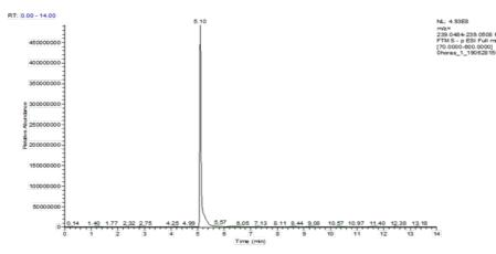
**Figure 4.4.** Extracted ion chromatogram of bentazone molecular ion (m/z 239.0496, mass error  $\leq$  5 ppm) from a fortified agricultural wastewater sample.
