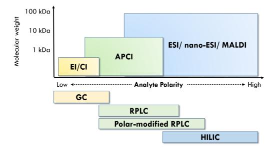
Figure 1.5. Instrumental capacity in terms of analyte polarity and molecular weight (based on Y. Wang et al., 2015)
