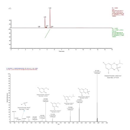
**Figure S7.** Extracted ion chromatograms (top: full MS, down: full MS<sup>2</sup>) and MS<sup>2</sup> spectrum of m/z 257.0238 (TP258).
