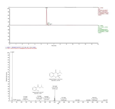
**Figure S13.** Extracted ion chromatograms (top: full MS, down: full MS<sup>2</sup>) and MS<sup>2</sup> spectrum of m/z 434.0869 (TP435).
