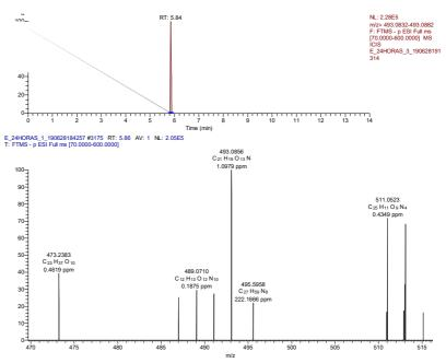
Figure S20. Extracted ion chromatogram and full MS spectrum of *m*/*z* 493.0856 (TP494).
