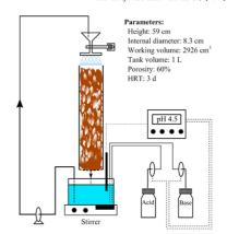
Fig. 1. Schematic representation of the experimental TBR set-up. HRT, hydraulic retention time.
