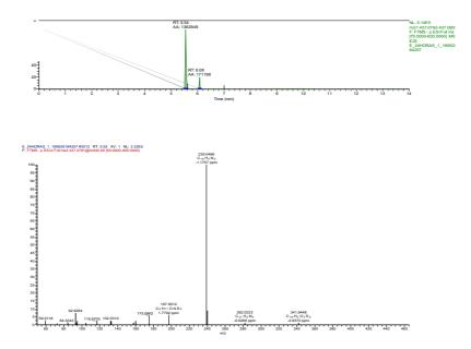
Figure S9. Extracted ion chromatogram and  $MS^2$  spectrum of m/z 437.0781 (TP438).
