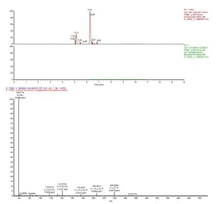
**Figure S17.** Extracted ion chromatograms (top: full MS, down: full MS<sup>2</sup>) and MS<sup>2</sup> spectrum of m/z 387.1225 (TP388).
