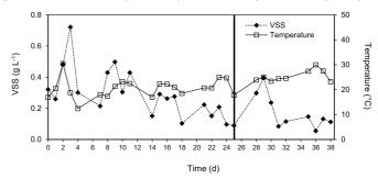
Fig. 2. Evolution of biomass concentration (VSS) and temperature in the pilot-PBR (HRT = 8 d). The vertical black line indicates the beginning of the steady-state.
