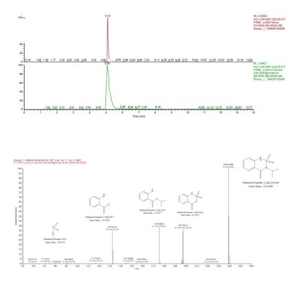
Figure S2. Extracted ion chromatograms (top: full MS, down: full MS<sup>2</sup>) and MS<sup>2</sup> spectrum of m/z 239.0496 (bentazone).
