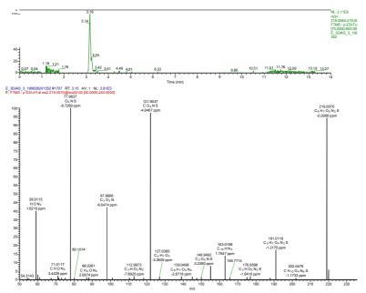
Figure S16. Extracted ion chromatogram and MS<sup>2</sup> spectrum of *m/z* 219.0070 (TP220).
