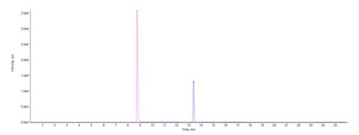
**Figure 4.3.** Extracted ion chromatogram of acetamiprid molecular ion (pink coloured peak, m/z 223.0745, mass error  $\leq$  5 ppm) and propanil molecular ion (blue coloured peak, m/z 218.0134, mass error  $\leq$  5 ppm) from a fortified sample.
