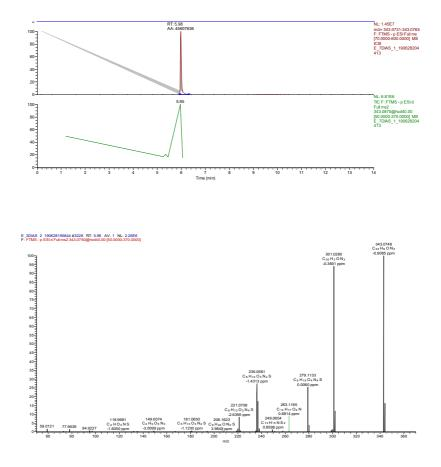
**Figure S10.** Extracted ion chromatograms (top: full MS, down: full MS<sup>2</sup>) and MS<sup>2</sup> spectrum of m/z 343.0748 (TP344).
