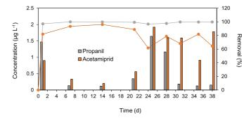
Fig. 4. Evolution of acetamiprid and propanil concentration in the pilot-PBR effluent (bar chart) and their removal efficiency (line chart).
