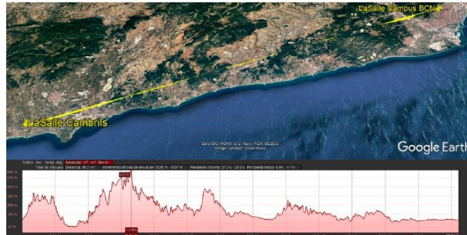
Figure 5. NVIS link between LaSalle Campus, BCN and Cambrils, Tarragona. The highest peak is located at 573 m above sea level.
