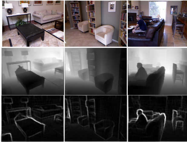
Figure 8.5: colour images (Row 1), associated depth images (Row 2) and their corresponding CS images (Row 3).
