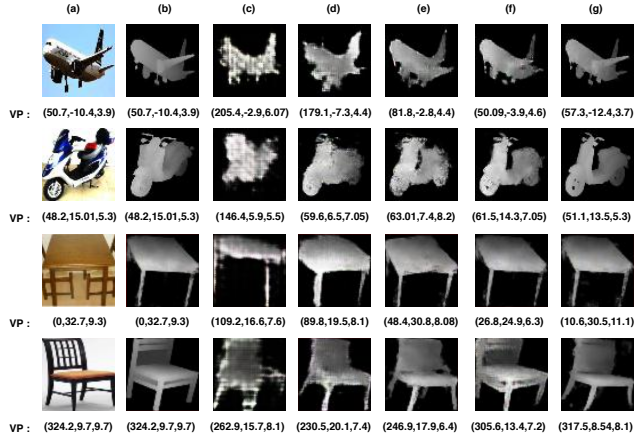
Figure 4.11: Example of depth predictions with our model. In each row, we show (a) input image, (b) ground truth, (c) output at epoch 100, (d) output at epoch 400, (e) output at epoch 1000, (f) output at epoch 1500, (g) output at epoch 2000 (final generated depth image). All images with the corresponding estimated viewpoints (VP), including (Azimuth and Elevation angles and Distance between object and camera). More results with the proposed model are given in the supplementary material.
