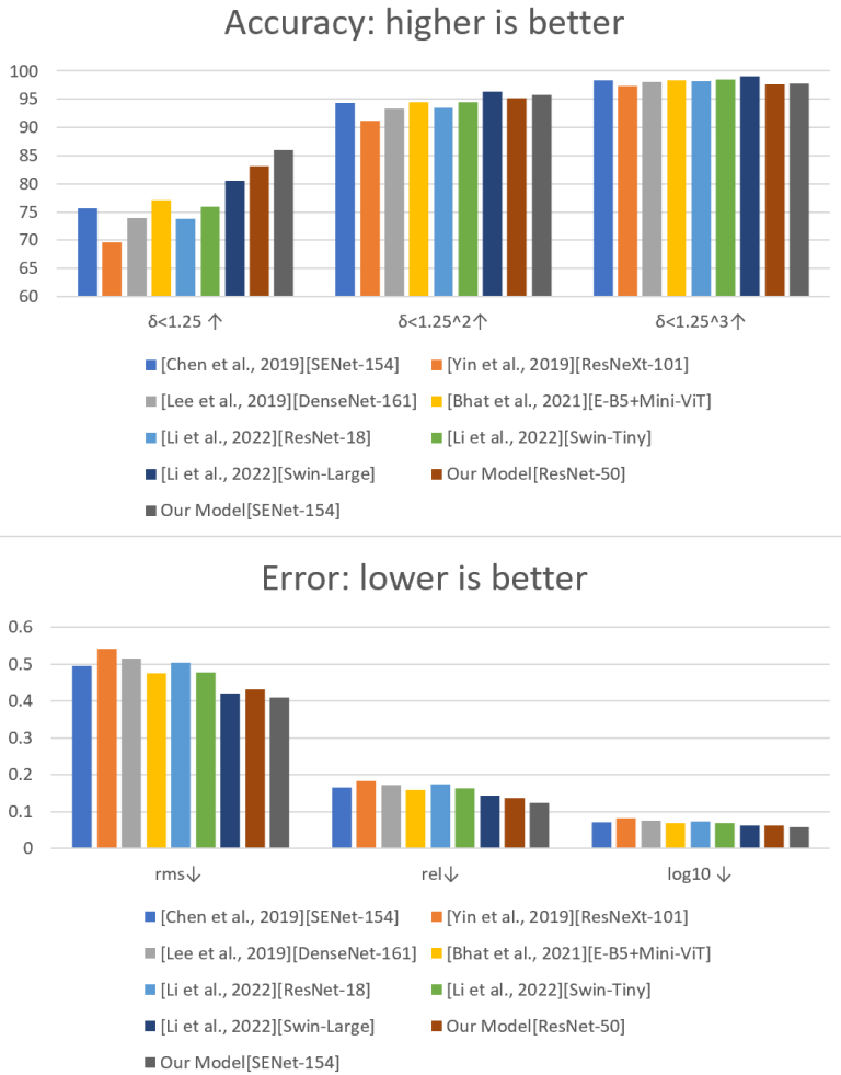
Figure 9.8: The accuracy and the three error measures of the five state-of-the-art models with our mode in the SUN RGB-D dataset.
