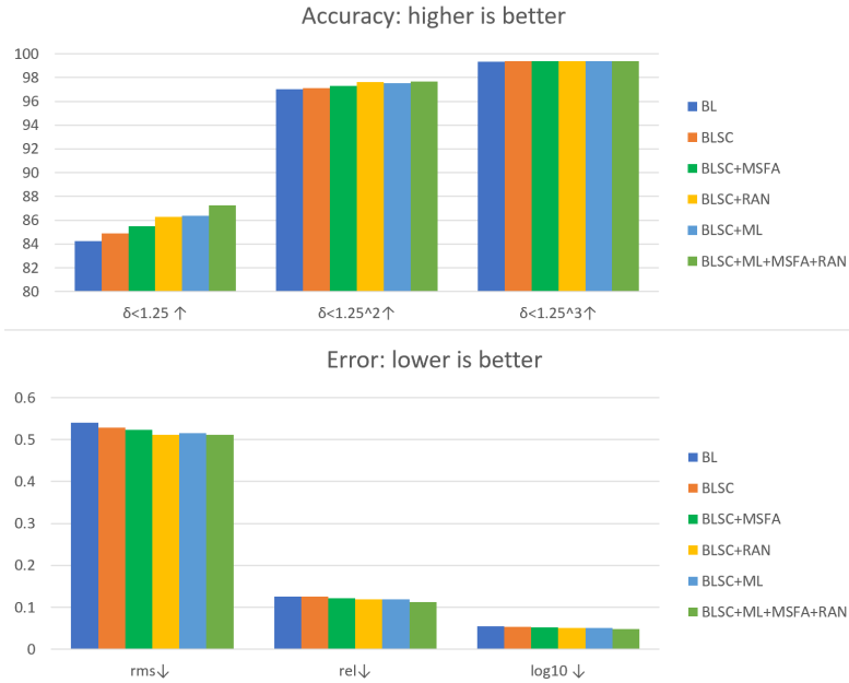
Figure 9.5: The accuracy and the three error measures of the six variations of our model with the NYU Depth-v2 dataset.
