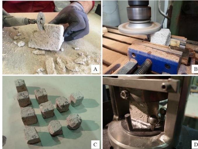
Fig. 48 Mortar specimen manufacturing process from the existing historical building 'Hi/I 4 '. A) Carving mortar cubes from amorphous collected samples. B) Dry polishing with a 3-axis vertical milling machine fitted with a rotary diamond disc. C) 40 × 40 × 40 mm 3 cubes specimens obtained. D) Cube specimen tested in a hydraulic press
