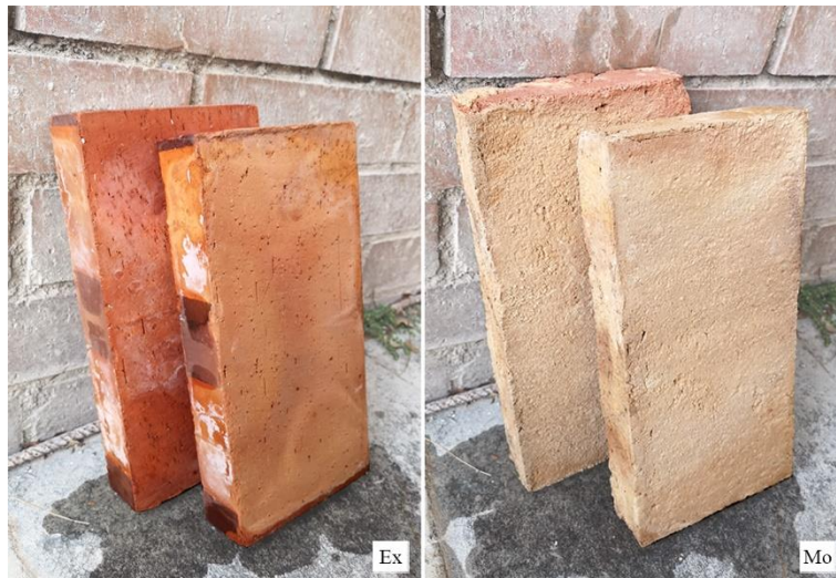
Fig. 24 Modern mechanically extruded solid fired clay brick ('Ex') (left), modern handmade solid fired clay brick ('Mo') (right)
