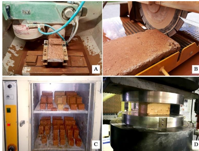
Fig. 15 Manufacturing process of the specimens: A) the grinder equipped with a rotary disc to polish the bricks until obtaining a constant thickness; B) the table saw equipped with a water jet to cut the specimens; C) the specimens in the oven at a constant temperature of 105 \pm 5 °C for 24 hours; D) 100 \times 100 \times 40 mm 3 specimen tested in the hydraulic press
