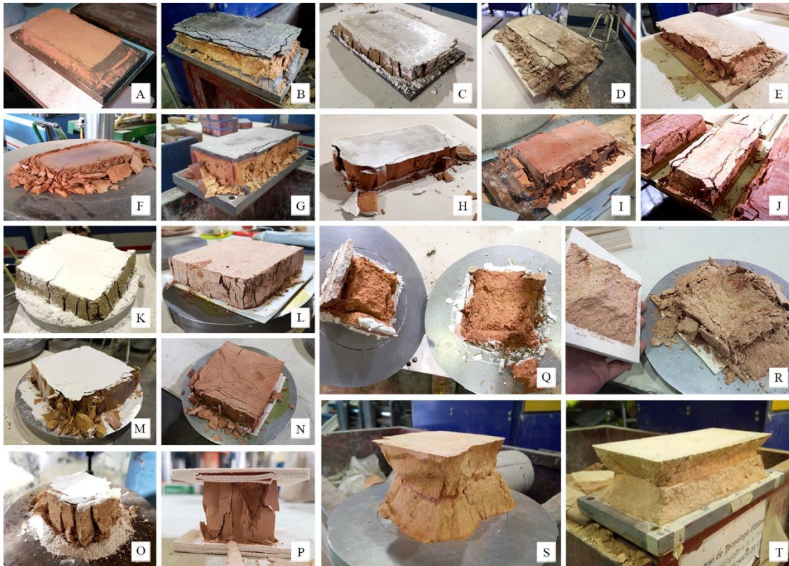
Fig. 27 Observed failure modes in the specimens with all bearing surface types. Handmade bricks 'Mo' from A) to E), K), L), O), Q), and R). Mechanically extruded bricks 'Ex' from F) to J), M), N), P), S), and T). A) and F) grinded, B) and G) capped with cement mortar, C) and H) capped with gypsum plaster, D) and I) placed with sheets of plywood, E) and J) placed with sheets of fibreboard, K) and M) covered with gypsum powder, L) and N) placed with two oiled PTFE leaves. O) 'Mo' 'C40' covered with gypsum powder, P) 'Ex' 'C40' placed with sheets of plywood, Q) 'Mo' '100' capped with gypsum plaster, R) 'Mo' '100' placed with plywood sheets, S) 'Ex' '2ha' grinded and stacked, T) 'Mo' '2wh' grinded and stacked
