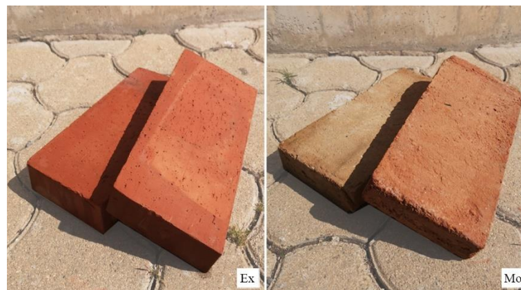
Fig. 34 Modern mechanically extruded solid fired clay brick (‘Ex’) (left), modern handmade solid fired clay brick (‘Mo’) (right)
