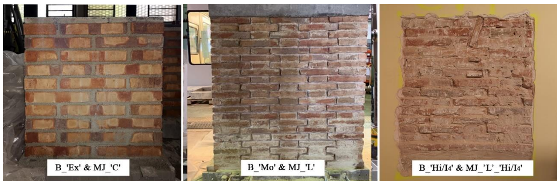
Fig. 46 Masonry walls manufactured with modern mechanically extruded solid fired clay brick and cement mortar (B_‘Ex’ & MJ_‘C’) (left), with modern handmade solid fired clay brick and lime mortar (B_‘Mo’ & MJ_‘L’) (centre), with historical handmade solid fired clay brick and lime mortar (B_‘Hi/I 4 ’ & MJ_‘L_‘Hi/I 4 ’) (right)
