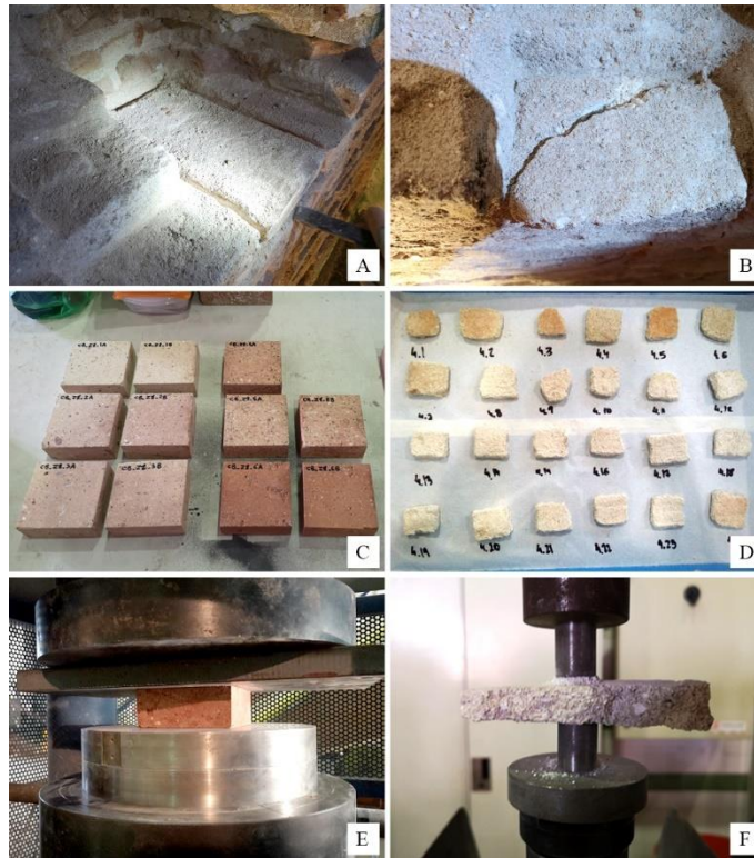
Fig. 47 Sample collection procedure in historical existing building, preparation of the specimens, and testing procedures. A) Extraction of the brick sample from existing wall, B) extraction of the mortar joint from existing wall, C) 100 x 100 x 40 mm 3 brick specimens prepared to be tested, D) mortar joint specimens prepared to be tested, E) brick specimen testing configuration, F) mortar joint testing configuration
