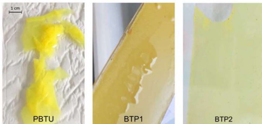
Figure S1. Photos of binding gels made from three polymeric materials derived from benzoylthiourea (PBTU, BTP1 and BTP2) mixed with a polyacrylamide gel solution at a ratio of 2.3% w/v
