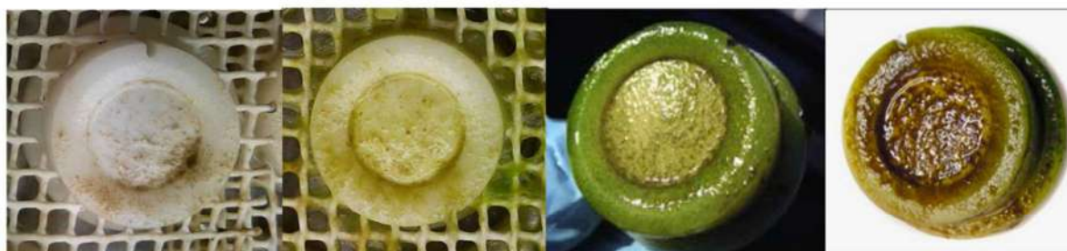
Fig. 3 Growth of biofilm in diffusive gradients in thin film devices deployed for several days in a eutrophic river water. Last picture shows biofilm and suspended particulate matter clogging the filter
