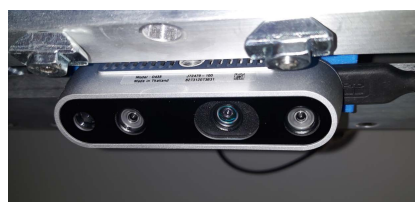
FIGURE 29. Intel RealSense D435, also used in the experiments, installed in the train inspection monorail wagon. The D435 model, compared to D415, has a wider field of view (FOV) and a global shutter.
