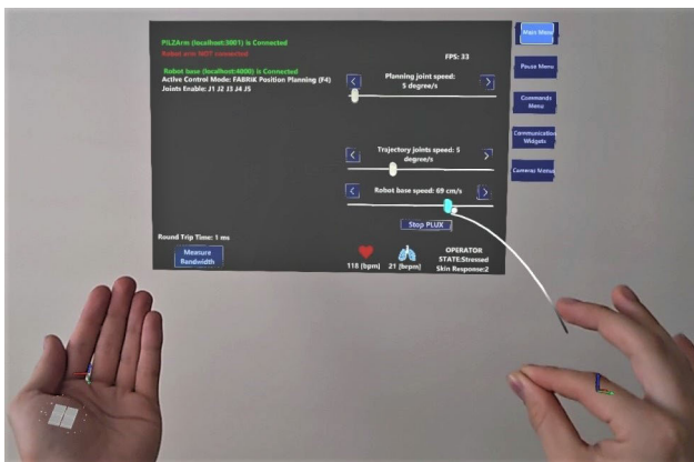
FIGURE 30. The hand menu opened by rotating the hand up and interacting with the right hand to change the speed of the robot base. The interaction can also be done using voice recognition or eye tracking and dwell.
