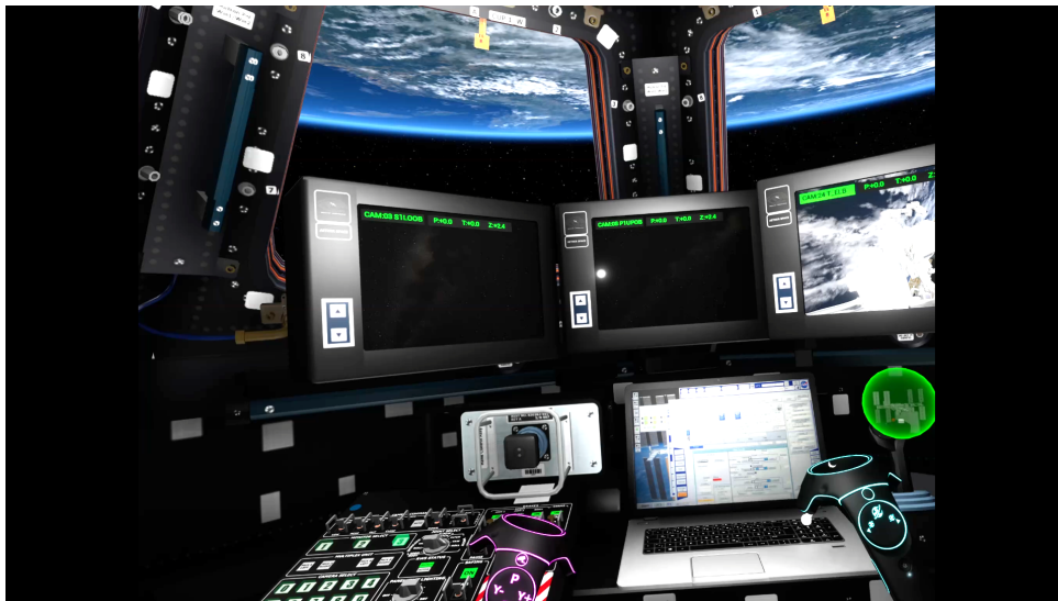
FIGURE 6.2: The International Space Station (ISS) robotic arm simulator from the Cupola observatory module. The work done by the author was focused on integrating the real robotic arm controllers in Mixed Reality.
