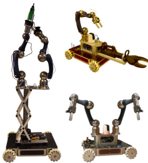
FIGURE 4. CERNBots with different configurations (dual or single manipulator, PTZ cameras, lifting stage, cutters, gripper or custom-made tools).
