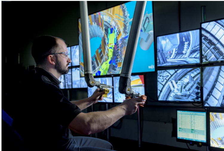
FIGURE 1.1: The MASCOT master arms are operated to replace components in the Joint European Torus (JET) tokamak [5]. The interface is composed of multiple screens with camera video feedback and 3D models visualisation.
