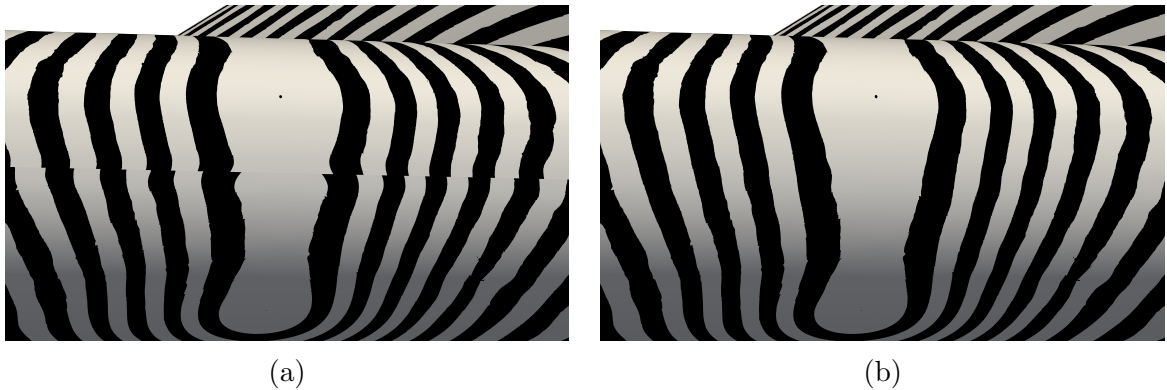
Figure 3.12: Close-up view of the leading edge of a Falcon aircraft wing. Zebra mapping on the mesh of polynomial degree four with (a) the initial model, and (b) the final model with the leading edge smoothed.
