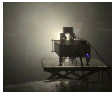
Figure 7.16: (Left) DoAPC with the active illumination in the fog chamber. (Right) Camera-illumination system working during a fog cycle inside the chamber.
