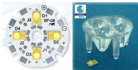
Figure 3.20: (Left) Picture of the white LEDs array. (Right) Image from the datasheet of the plastic lenses that collimate the light emitted by the LEDs
