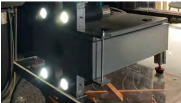
Figure 7.16: (Left) DoAPC with the active illumination in the fog chamber. (Right) Camera-illumination system working during a fog cycle inside the chamber.
