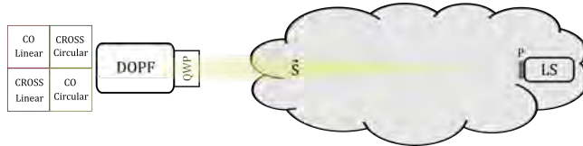
Figure 7.12: Scheme of the set-up for detection in the transmission of forward-scattered light from fog under active illumination. The light source (LS) with the polarizer (P) illuminates the fog with polarization \vec{S} that is forward scattered to the modified DoFP camera at 28 m.
