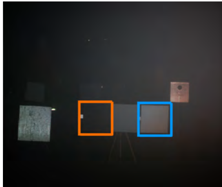
Figure 7.10: Calibrated diffusive panels for embedded object detection in fog. The two panels of interest are highlighted: a black panel of 0% reflectance in orange and a white panel of 100% reflectance in blue.
