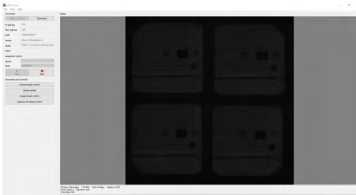
Figure 3.17: Frame grabber software: visualization menu of the eBUS Player to see the raw acquisitions. Four sub-images are distinguished corresponding to the four configurations of the retarders in the RA.
