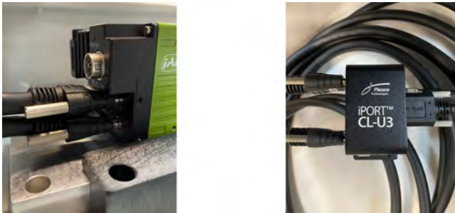
Figure 3.13: (Left) Camera Link connectors (PMCL). (Right) iPORT CL-U3 frame grabber with the PCML coming from the sensor on the left side and the USB 3.0 on the right side to connect to the PC.
