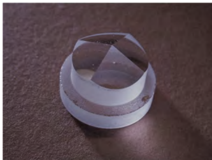
Figure 3.1: The glass pyramid used on the William Herschel telescope [170]. Note that its diameter is no more than 15 mm.
