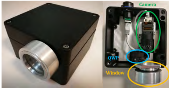
Figure 7.3: (Left) Enclosed camera into an IP68 housing cage to preserve the seal of the inner cavity. (Right) Set-up of the modified DoFP camera together with the QWP aligned to the horizontal axis.
