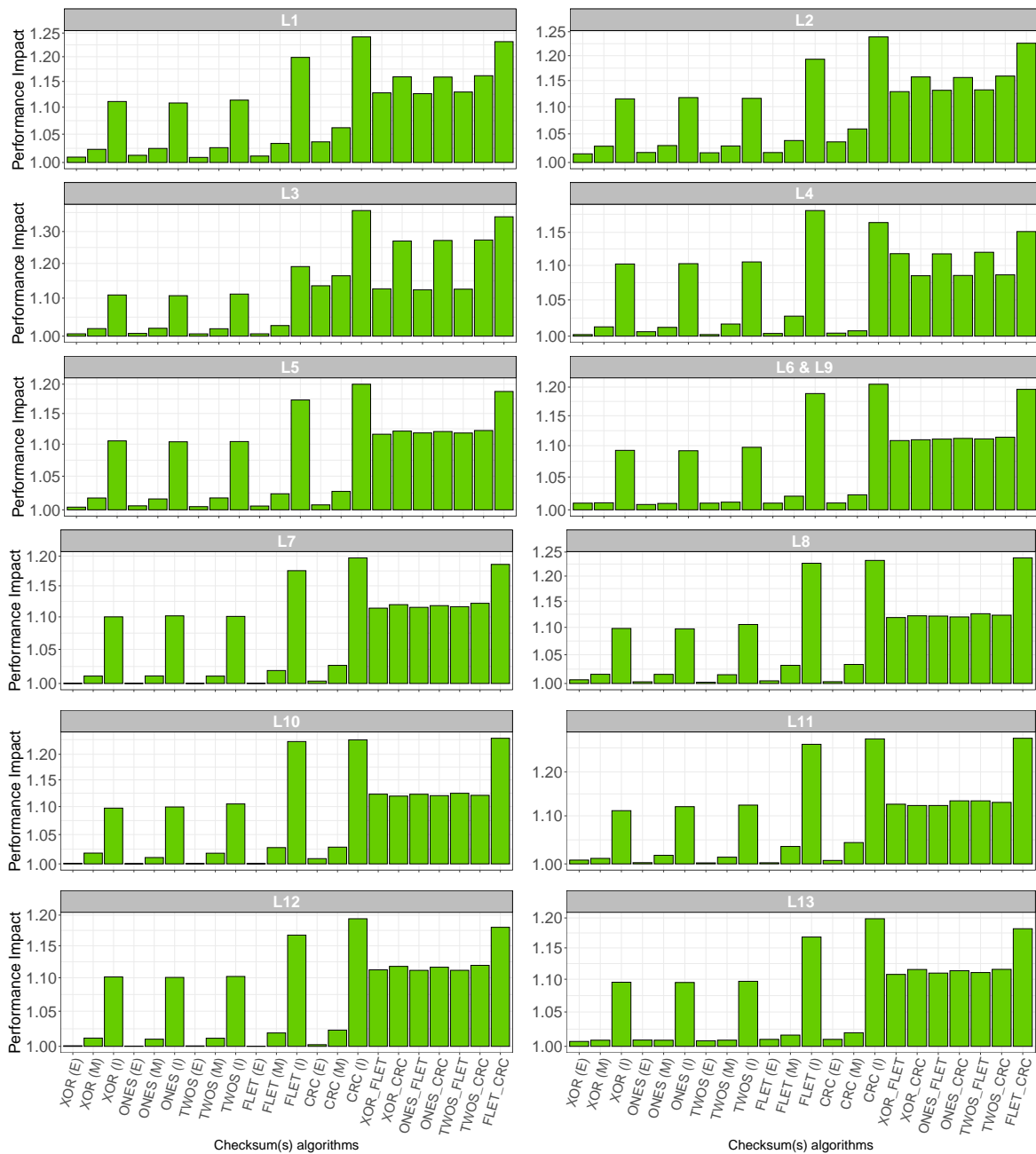
Fig. 6.4: Layer-by-layer performance impact without compiler optimizations (-O0)
