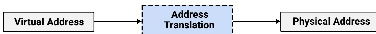
Figure 2.7: The fundamental idea behind virtual memory systems → each memory access requires a translation from the virtual address space to the physical address space. Dotted lines indicate actions.
