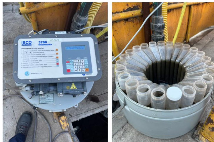
Figure 7.20 Automatic sampler: configuration panel (left) and interior of the sampler with 24 bottles for samples.
