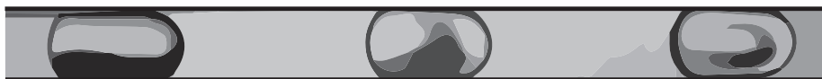
Figure 1.1: Snapshot of a microfluidics experiment inspired by [57]: three microdroplets, moving from left to right, containing dark-colored dye.
