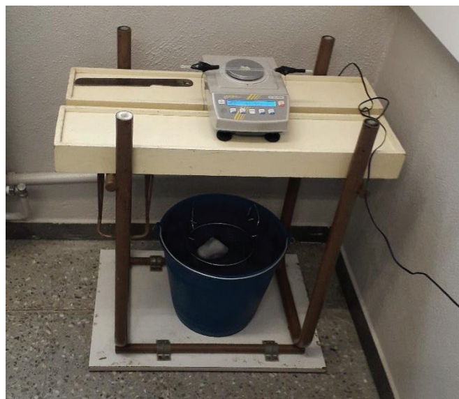
Figure 3.25 Hydrostatic bascule built with the laboratory material.
