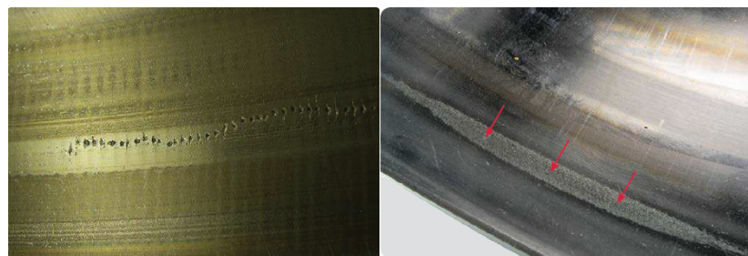
Figure 6. Electrical erosion failures. Excessive current (left) and current leakage (right) [27]. Courtesy of SKF.
