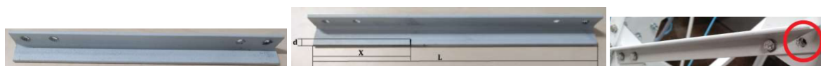
Figure 3. Different structural state scenarios studied in this work. Replica (healthy) bar (left). Crack damage, where L is the length of the bar, d = 5 mm is the crack size, and X = L/3 is the location of the crack in the bar (center). Missing bolt (right).
