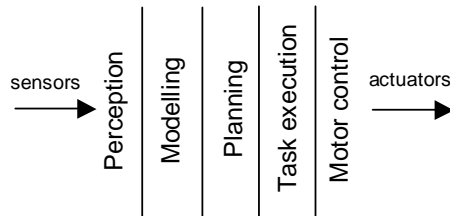
Figure 2.1: Phases of a classical deliberative control architecture.
